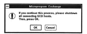
(7-2) It is necessary to switch the SCSI path to the alternate path before executing the microprogram FC for the CHA (SCSI) PCB. To continue the processing, select (CL) [Yes]. Go to step (8).
