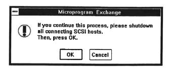
(3-2) It is necessary to switch the SCSI path to the alternate path before executing the microprogram FC for the CHA (SCSI) PCB. To continue the processing, select (CL) [Yes]. Go to step (4).
