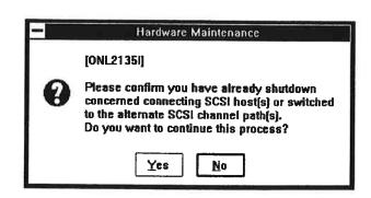
This processing is a special procedure for detecting a cause of a bus error. Contact the technical support center before performing this processing.
