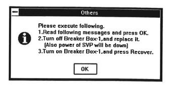
6. The message shown on the right is displayed. (Reply with [OK] after performing the hardware procedure.)
