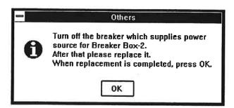
7. When redundant power supply is installed. "Do you want to replace the "Breaker Box-n?"" is displayed.
