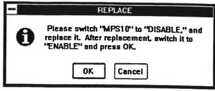
When replace 5VPSx0 or 5VPSx1, if target PS is normal and other 5VPSs are in failure, the message shown on the right is displayed.
