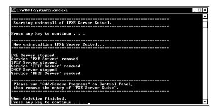
(18) The message "End of the uninstall of [PXE Server Suite] and [Setup on SVP]." appears. When the message "Press any key to continue..." appears, press any key.
