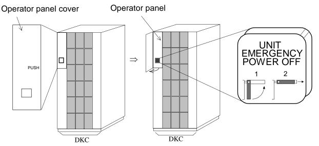
Fig. 1.2-1 Operation of UNIT EMERGENCY POWER OFF switch
