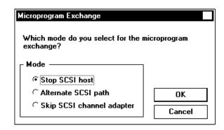
• "Stop SCSI host": Exchange micro-programs by varying off-line the SCSI host paths.
