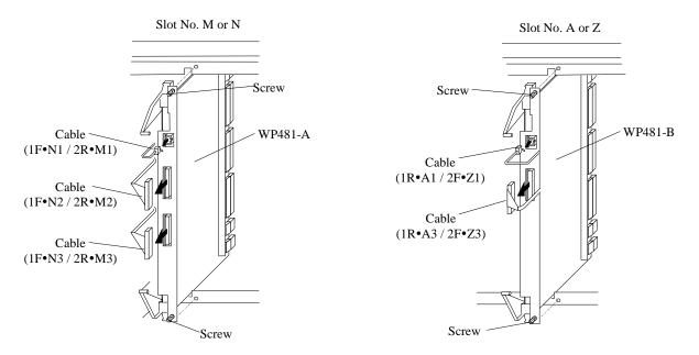
3. Insert the spare PCB to the correct location and fasten the screws.
