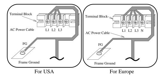
Fig.T17-9 Connection of AC Power Cables to the Terminal Block
