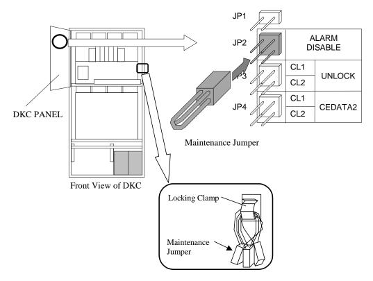
Fig. T29-1 Connection of Alarm INH Jumper
