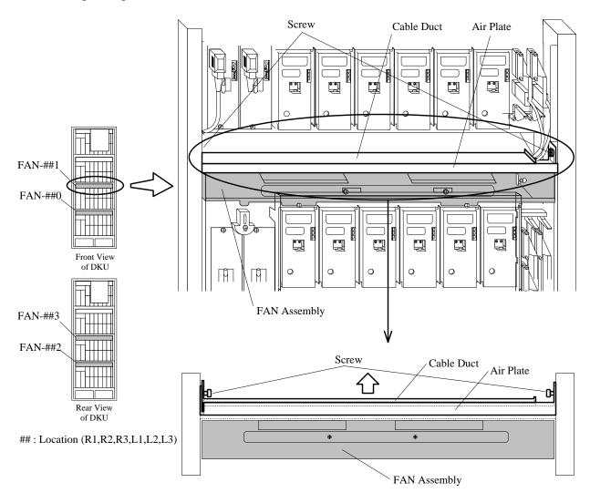
Fig. FT4-1 Move the air plate(When FAN-##0 to FAN-##3 is replaced)
