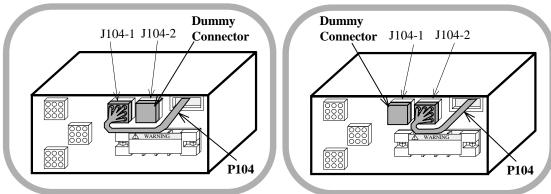
For USA (Input AC Voltage: 200 - 240V) For Europe (Input AC Voltage: 380 - 415V)
