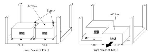
Fig. FT5-4 Removal of AC BOX
