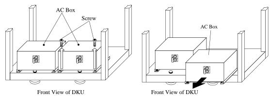
Fig. FT6-4 Removal of AC BOX
