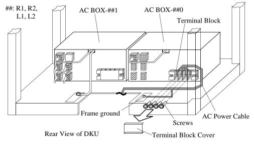
Fig. T30-3 Disconnection of AC Power Cable
