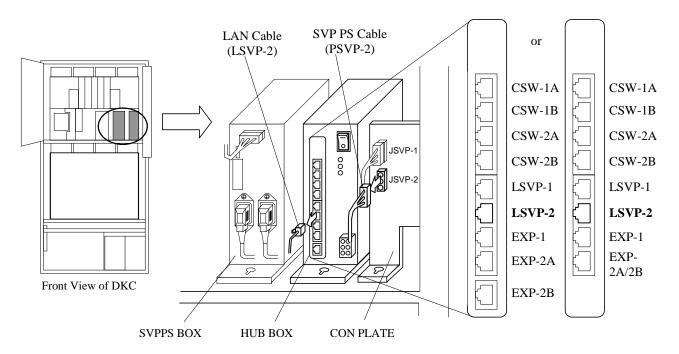
Fig. T7.1-9 Disconnect of LAN Cable and SVP-PS Cable
