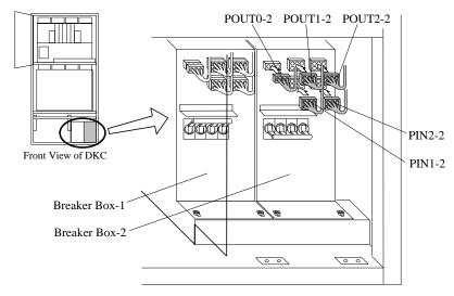
Fig. T10-7 Connection of Cable Connectors
