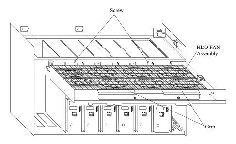
Fig. FT4-3 Removal of HDD FAN Assembly
