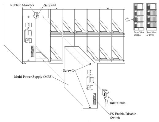
Fig. FT3-1 Replacement of Multi Power Supply
