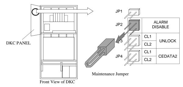
Fig. T21-10 Disconnection of Jumper
