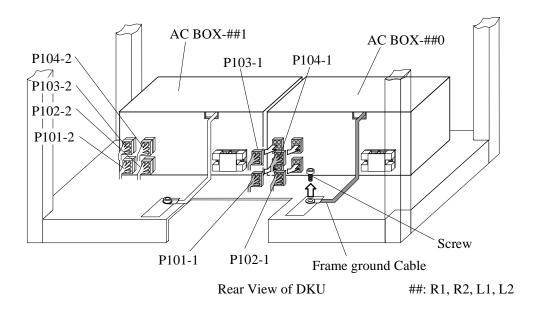
Fig.T22-8 Connection of Cables
