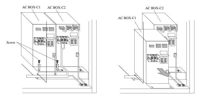
Fig. T21-5 Removal of AC BOX
