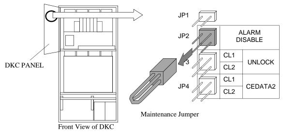
Fig. T10-9 Disconnection of Jumper
