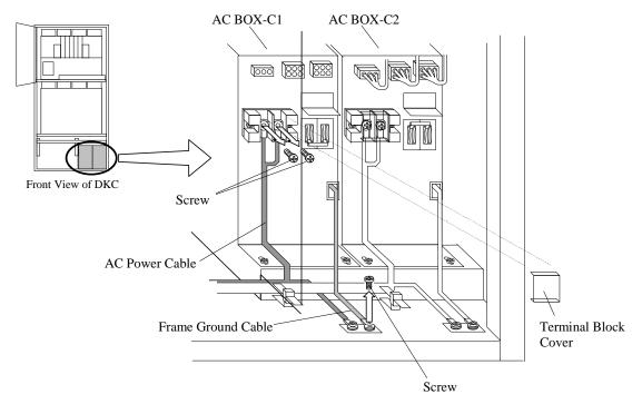
Fig. T21-4 Removal of AC Power Cables
