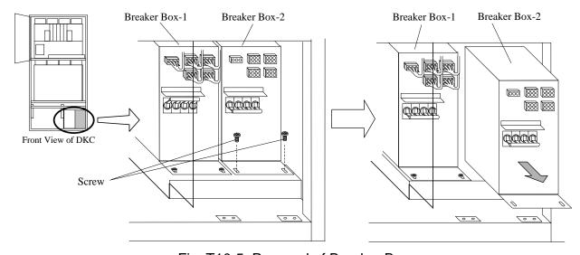
Fig. T10-5 Removal of Breaker Box
