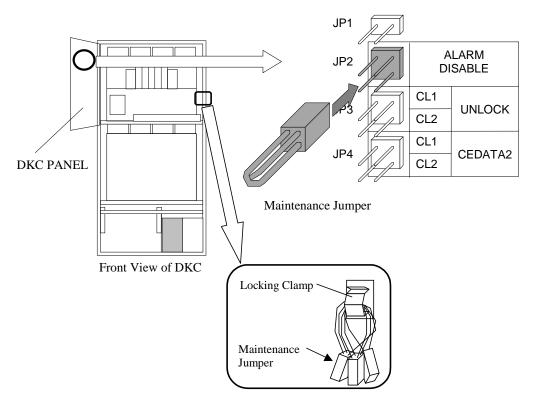
Fig. T9-1 Connection of Alarm INH Jumper
