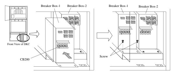
Fig. T9-6 Attachment of Breaker BOX
