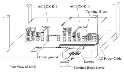
Fig. T17-5 Disconnection of AC Power Cable
