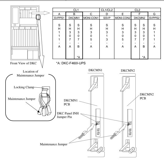
Fig. T2-1 Insertion of Maintenance Jumper
