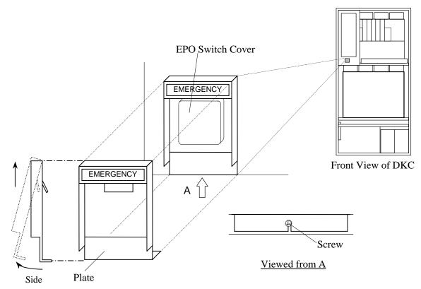
Fig. T2-2 Removal of Plate
