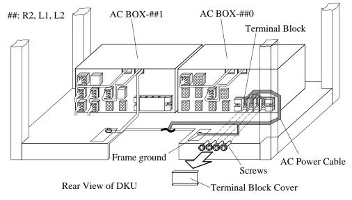
Fig. T18-3 Disconnection of AC Power Cable
