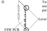
Two types of levers for inserting/removing the FSW, large and small ones, are used. The levers were enlarged to make the operation easier, accordingly their performance and function are the same.
