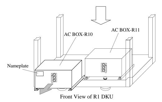
Fig. T17-6 Removal of AC BOX
