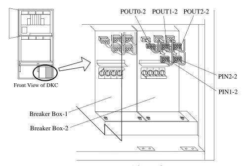
Fig. T10-4 Removal of Cable Connector
