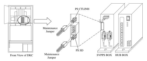
Fig. T7.1-4 Jumper settings of SVPPS BOX
