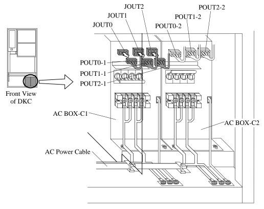
Fig. T29-3 Removal of Cable Connector
