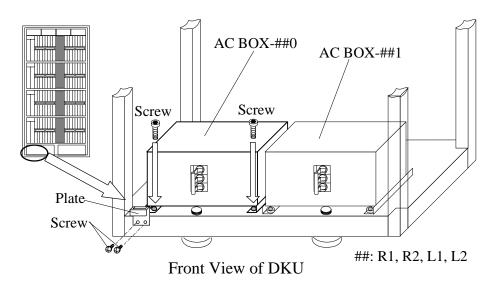
Fig. T22-6 Attachment of AC BOX
