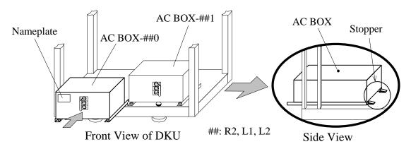
Fig. T18-5 Installation of new AC BOX
