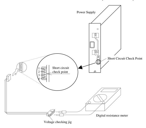
Fig. T13-2 Short Circuit Check Point
