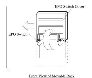
Fig. T1-3 Removal of EPO Switch Cover
