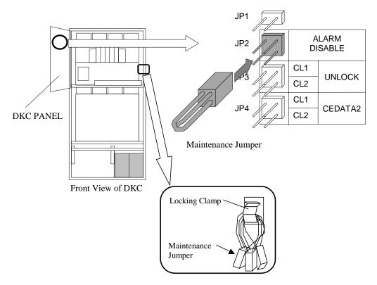
Fig. T21-1 Connection of Alarm INH Jumper
