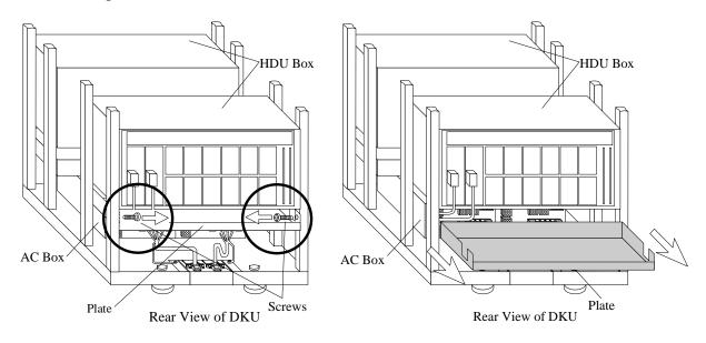
Fig. FT5-2 Removal of Plate
