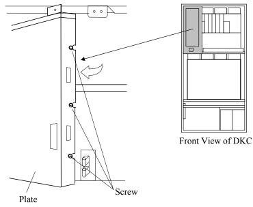
Fig. T1-4 Removal of Plate
