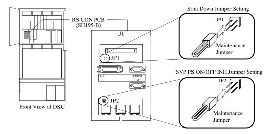
Fig. T7.1-3 Jumper settings of RS CON PCB
