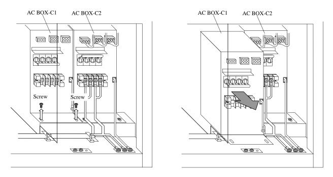
Fig. T29-5 Removal of AC BOX
