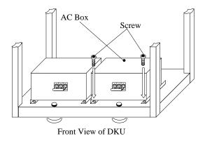
Fig. FT5-6 Attachment of spare AC BOX
