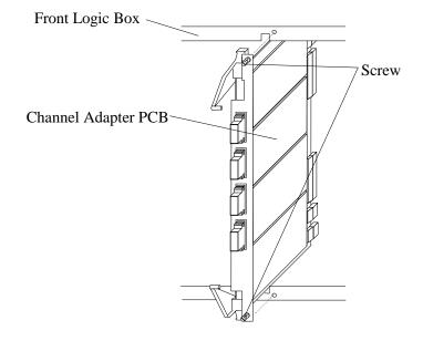
4. Insert the spare PCB to the correct location and fasten the two screws.
