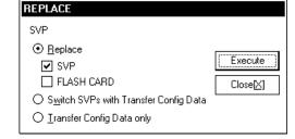
When you switch a Master SVP to a Standby SVP and vice versa, select (CL) [Switch SVPs with Transfer Config Data], and select (CL) [Execute].
