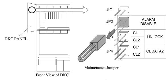
Fig. T29-10 Disconnection of Jumper
