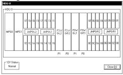
4. <Specify replacement on HDD> Make sure that the status is FAILED.
