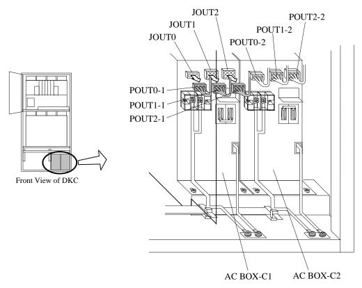
Fig. T21-3 Removal of Cable Connector
