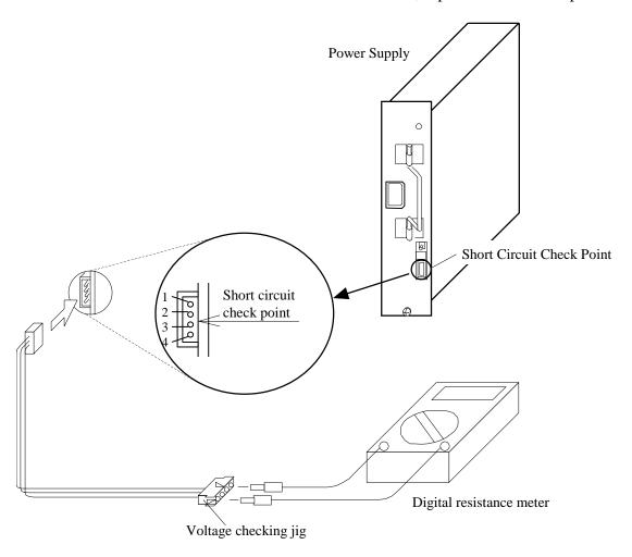
Fig. FT3-2 Short Circuit Check Point
