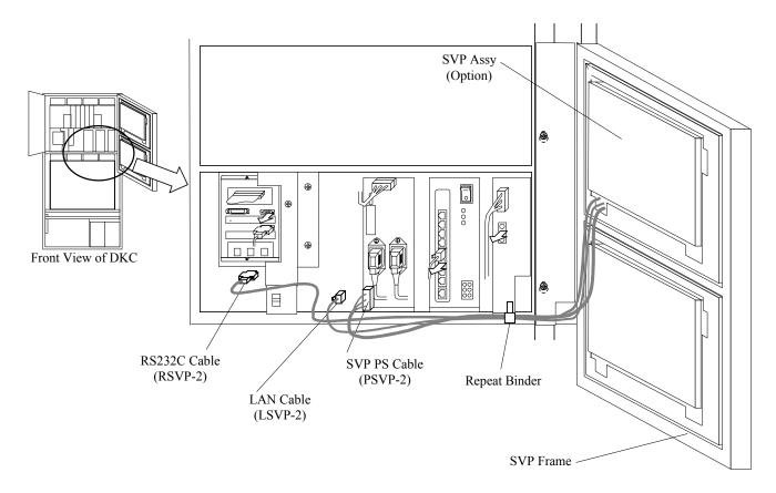
Fig. T7.1-10 Removal of Cables
