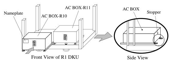
Fig. T17-7 Installation of new AC BOX
