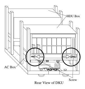
Fig. FT5-10 Attachment of Plate
