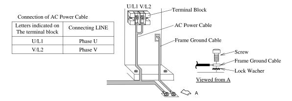
Fig. T21-7 Connection of AC Power Cable
