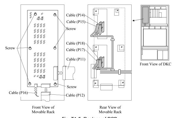
Fig. T1-5 Replace of PCB
