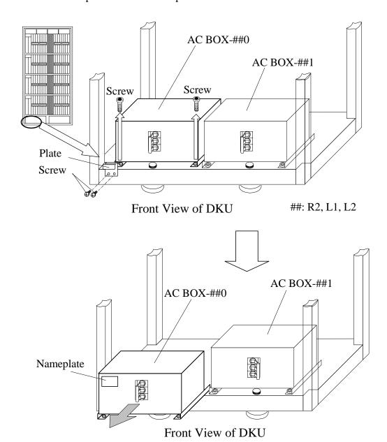
Fig. T18-4 Removal of AC BOX
