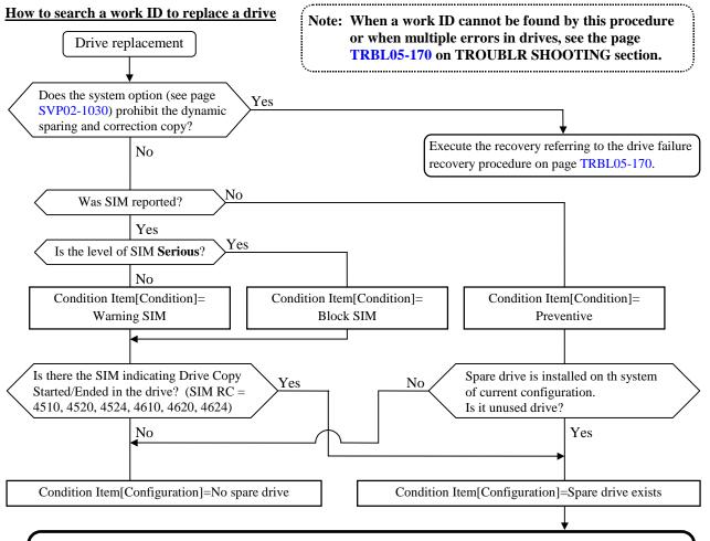
Search an appropriate Work ID from the Parts Replacement Process Table on REP01-150 according to the <u>Condition Item [Condition]</u> and <u>Condition Item [Configuration]</u> gotten in the above flowchart, and whether the drive to be replaced is installed in the position of spare drive or not.
