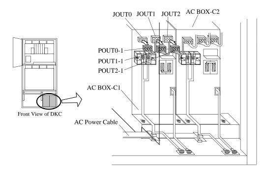
Fig. T21-8 Connection of Cable Connectors
