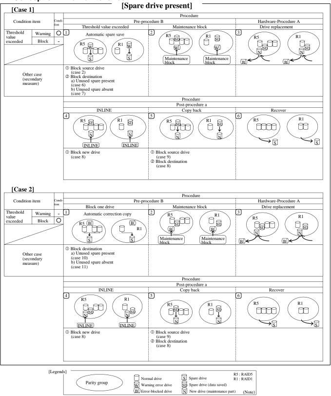
(Note) In RAID 1 method, Parity group consists of four drives.
