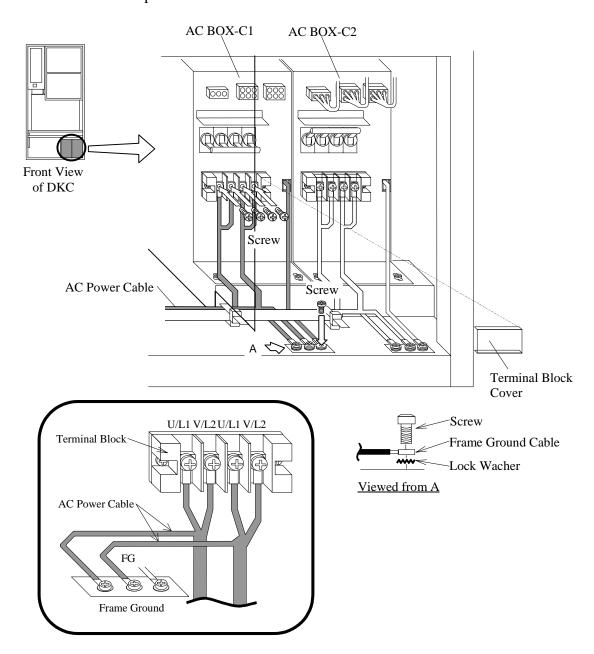
Fig. T29-7 Connection of AC Power Cable
