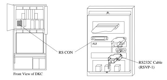
Fig. T7.1-5 Disconnect of RS232C Cable
