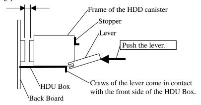
(2) Turn the lever at a stroke by pushing its top with your thumb.
