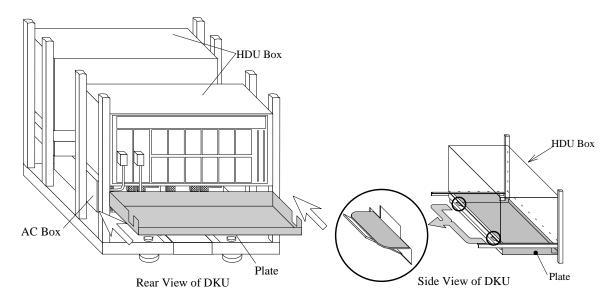
Fig. FT5-9 Attachment of Plate
