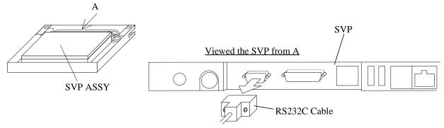
Fig. T7.3-3 Removing and installing RS232C Cable
