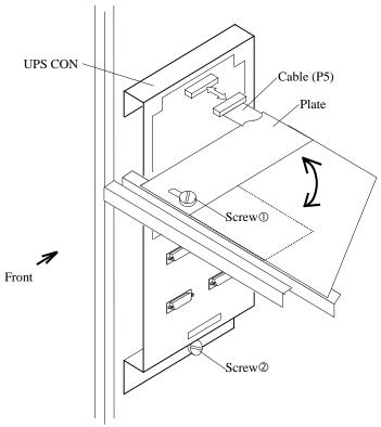
Fig. T27-2 Replacement of UPS CON
