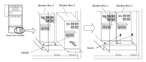
Fig. T10-6 Attachment of Breaker BOX
