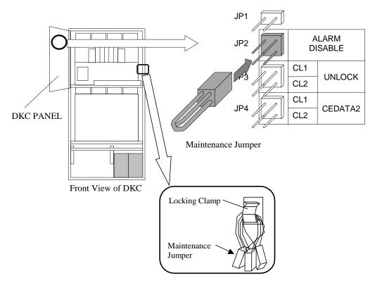
Fig. T17-1 Connection of Alarm INH Jumper
