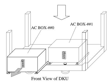
Fig. T31-4 Removal of AC BOX
