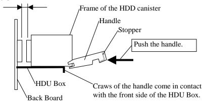
(2) Turn the handle at a stroke by pushing its top with your thumb. (Do not stop the handle on its way of turning.)
