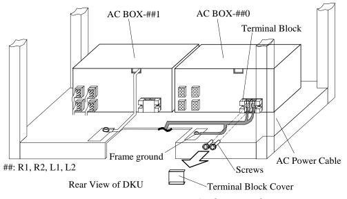
Fig. T22-3 Disconnection of AC Power Cable
