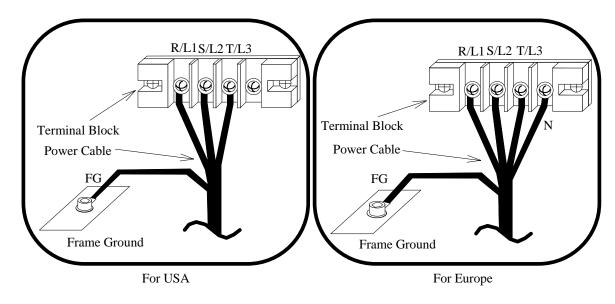
Fig. FT5-7 Connection of AC Power Cable to Terminal Block
