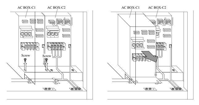
Fig. T28-5 Removal of AC BOX
