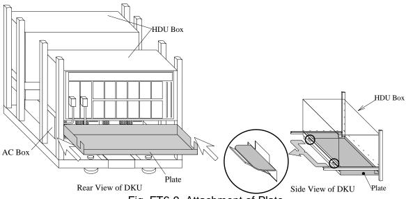
Fig. FT6-9 Attachment of Plate
