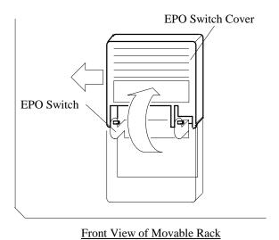
Fig. T2-3 Removal of EPO Switch Cover
