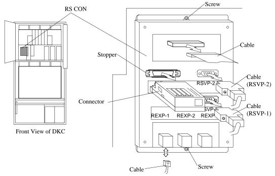
Fig. T19-1 Replacement of RS CON
