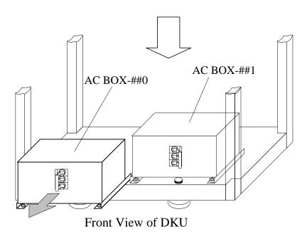
Fig. T30-4 Removal of AC BOX
