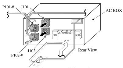
Fig. FT6-8 Connection of Cable Connectors
