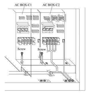
Fig. T28-6 Attachment of AC BOX
