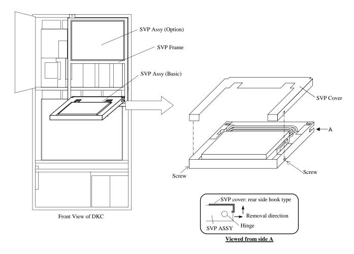
Fig. T7.1-11 Removing SVP cover
