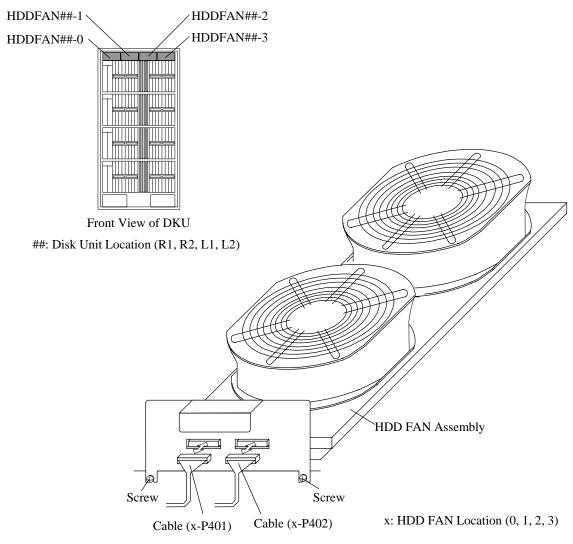
Fig. T16-1 Removal of HDD FAN Assembly
