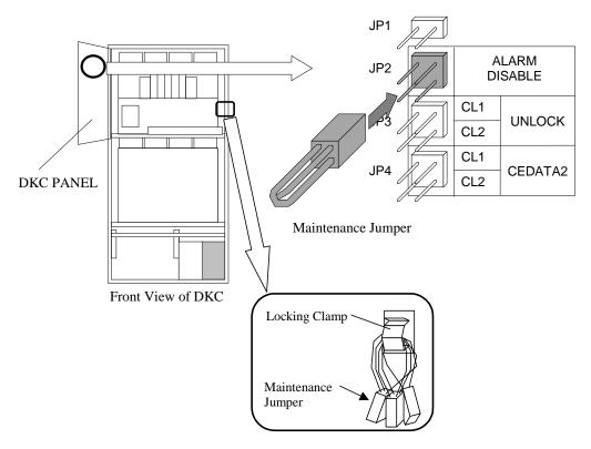
Fig. T10-1 Connection of Alarm INH Jumper
