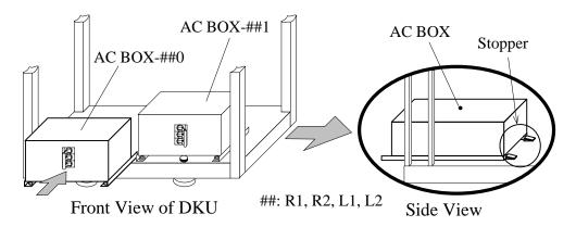
Fig. T30-5 Installation of spare AC BOX
