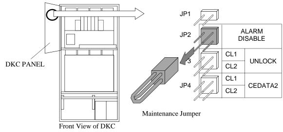
Fig. T9-9 Disconnection of Jumper
