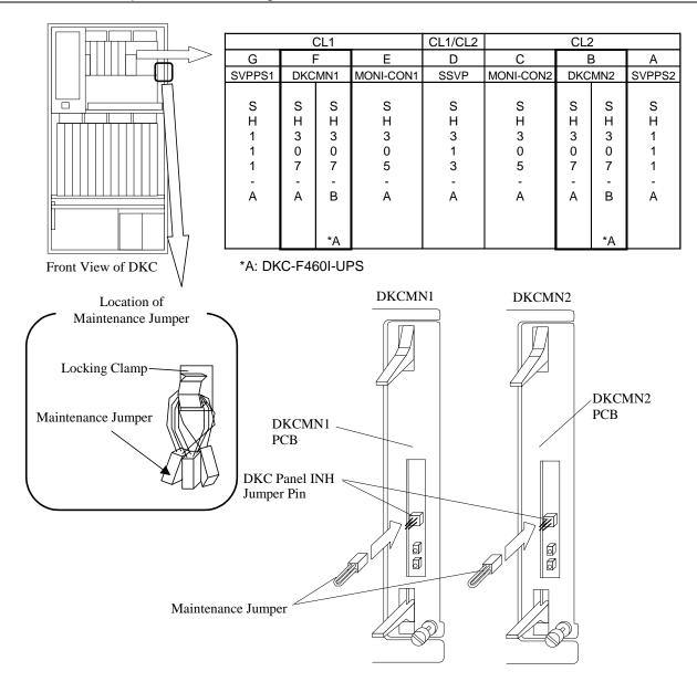
Fig. T1-1 Insertion of Maintenance Jumper
