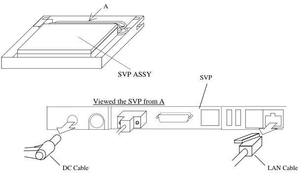
Fig. T7.3-1 Removing and installing Cables
