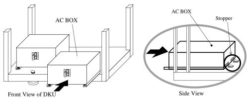
Fig. FT6-5 Spare AC BOX Installation
