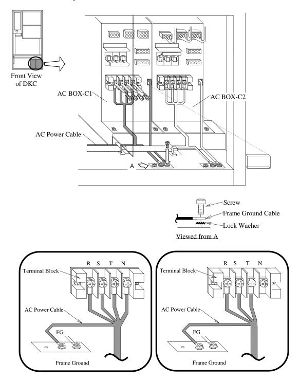
Fig. T28-7 Connection of AC Power Cable
