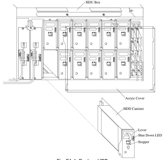
Fig. FA-1 Replace HDD
