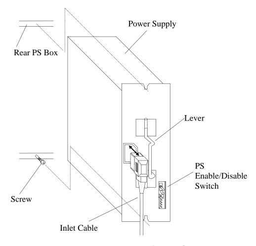
Fig. T13-1 Replacement of Power Supply
