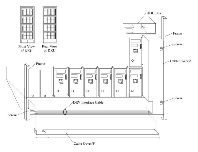
Fig. FT1-1 Removal of Cable Covers
