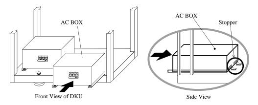
Fig. FT5-5 Installation of spare AC BOX
