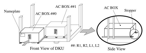
Fig. T22-5 Installation of new AC BOX
