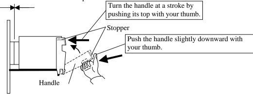
Fig. A-1 Method of Installing HDD Canister
