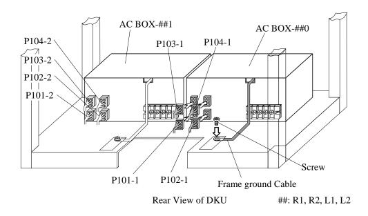
Fig.T31-8 Connection of Cables
