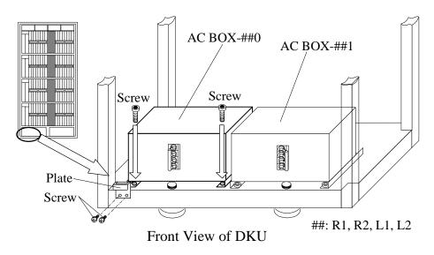
Fig. T31-6 Attachment of AC BOX
