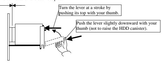
Fig. FA-2 Method of Installing HDD Canister
