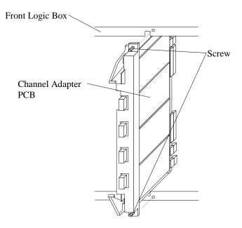
4. Insert the spare PCB to the correct location and fasten the two screws.
