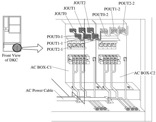
Fig. T29-8 Connection of Cable Connectors
