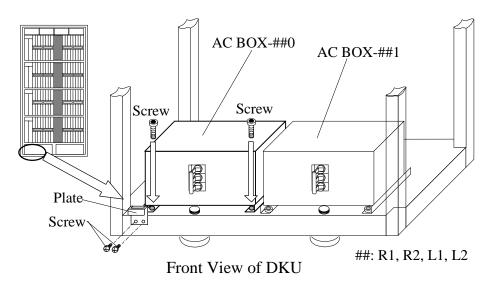
Fig. T30-6 Attachment of AC BOX
