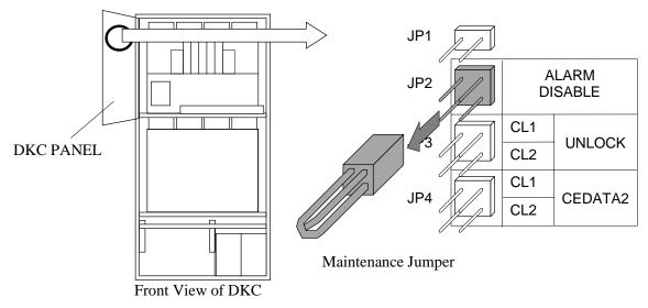
Fig. T17-12 Disconnection of Jumper
