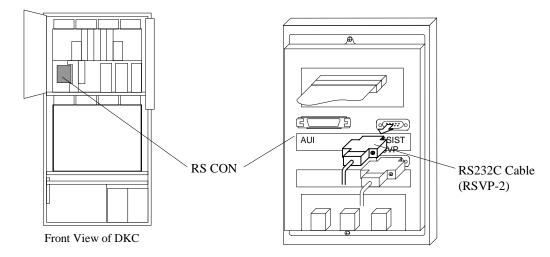
Fig. T7.1-8 Disconnect of RS232C Cable
