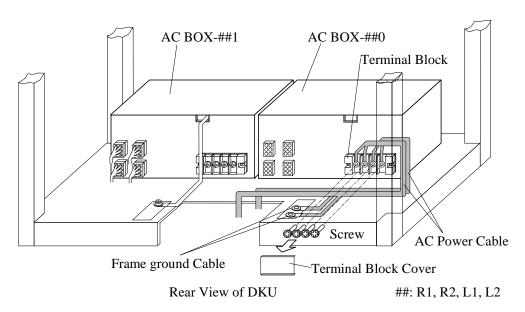
Fig. T31-3 Disconnection of AC Power Cables
