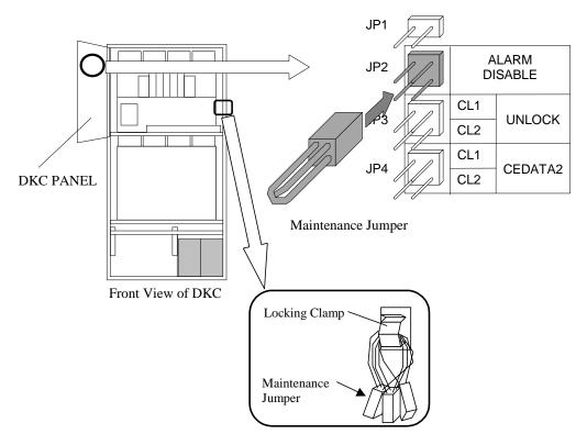
Fig. T28-1 Connection of Alarm INH Jumper
