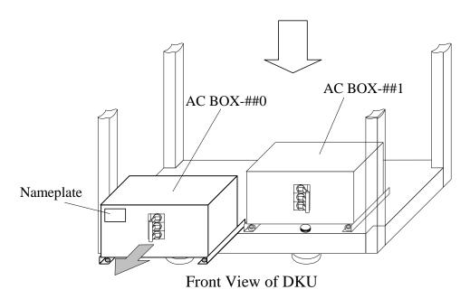
Fig. T22-4 Removal of AC BOX
