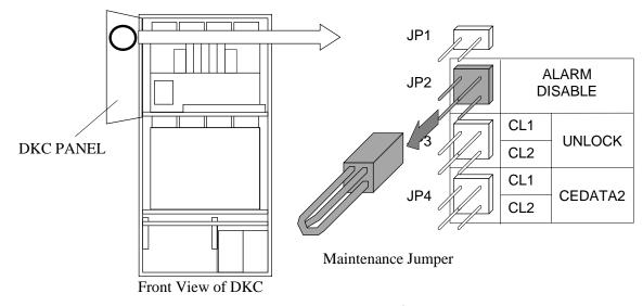
Fig. T28-10 Disconnection of Jumper
