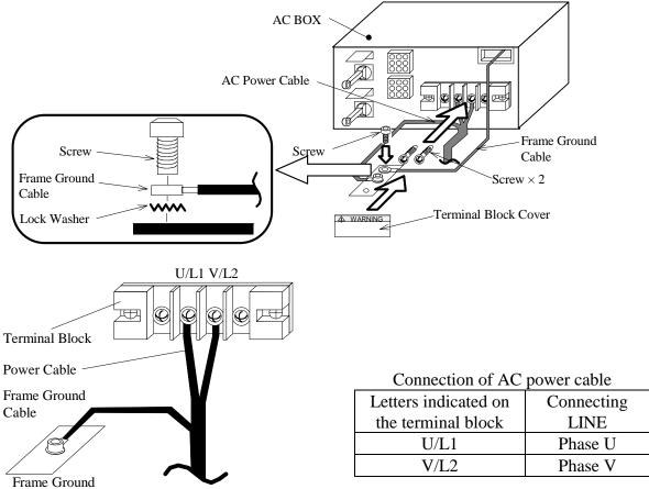
Fig. FT6-7 Connection of AC Power Cable
