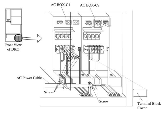
Fig. T29-4 Removal of AC Power Cables
