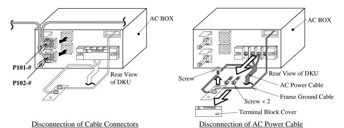
Fig. FT6-3 Disconnection of Cable Connectors and AC Power Cable
