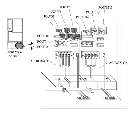
Fig. T28-3 Removal of Cable Connector
