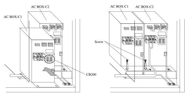
Fig. T21-6 Attachment of AC BOX
