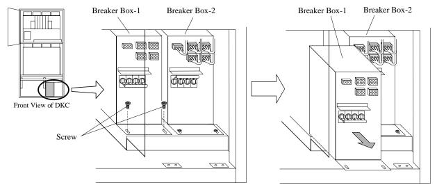
Fig. T9-5 Removal of Breaker Box
