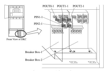
Fig. T9-7 Connection of Cable Connectors
