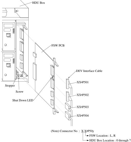
Fig. FT1-2 Replacement of FSW PCB
