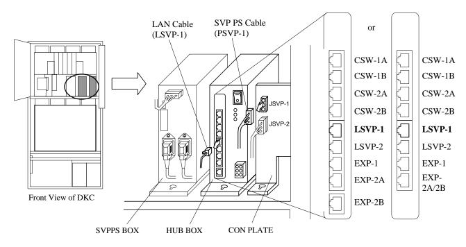
Fig. T7.1-6 Disconnect of LAN Cable and SVP-PS Cable
