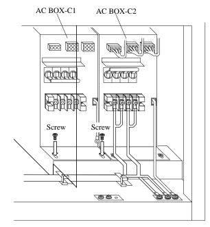
Fig. T29-6 Attachment of AC BOX
