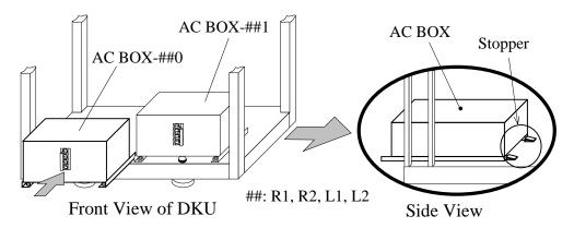
Fig. T31-5 Installation of Spare AC BOX
