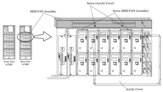
Fig. FT4-2 Removal of Acrylic Cover
