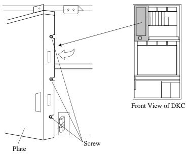
Fig. T2-4 Removal of Plate
