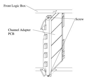
4. Insert the spare PCB to the correct location and fasten the two screws.
