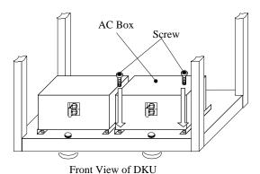
Fig. FT6-6 Spare AC BOX Installation
