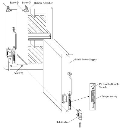
Fig. T15-1 Replacement of Multi Power Supply
