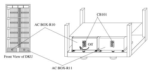
Fig. T17-3 Turn Off the Circuit Breaker of AC BOX
