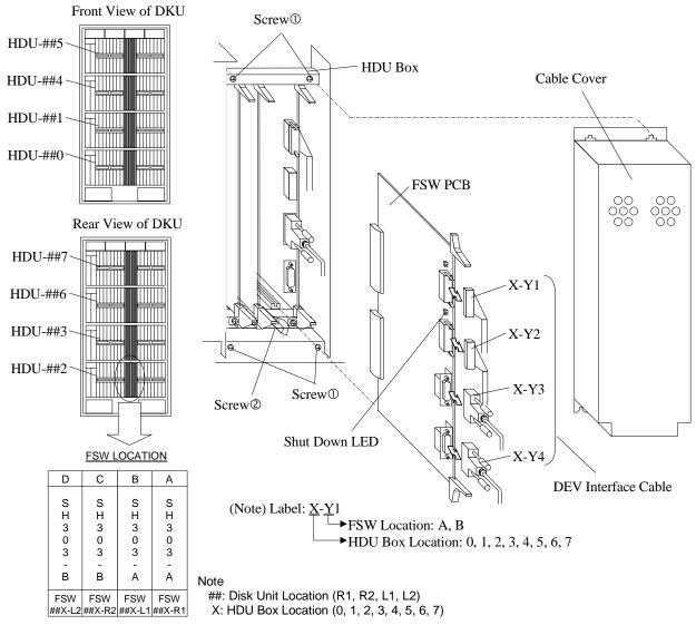
Fig. T20-1 Replacement of FSW PCB
