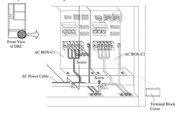
Fig. T28-4 Removal of AC Power Cable
