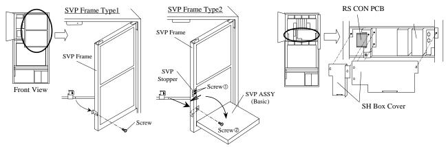
Fig. T19-1 Open the SVP Frame and remove the SH Covers
