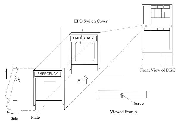
Fig. T1-2 Removal of Plate
