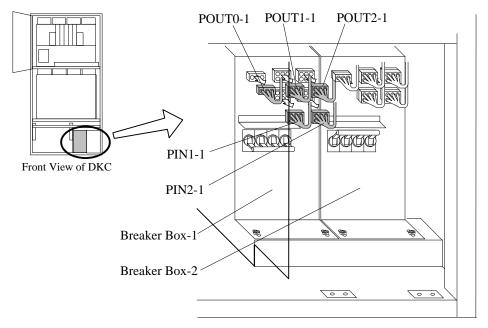
Fig. T9-4 Removal of Cable Connector
