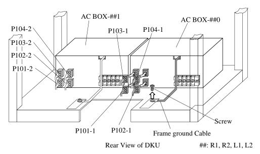
Fig. T31-2 Disconnection of Cable Connectors from AC BOX
