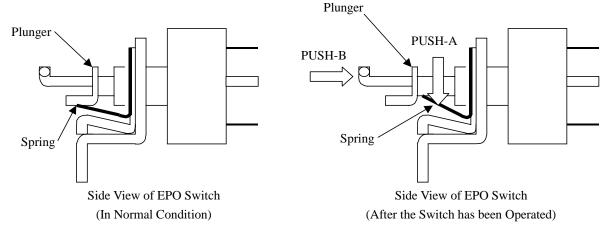
Fig. T1-6 Condition of the EPO switch
