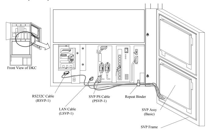
Fig. T7.1-7 Removal of Cables
