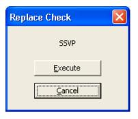
2. < Check beginning of special part Replacement> The message "RESTART switch, REMOTE MAINTENANCE switch and the environment check will be disabled. SVP-SSVP communication will be blocked. Do you want to replace the "SSVP?"" is displayed. Select (CL) [OK].
