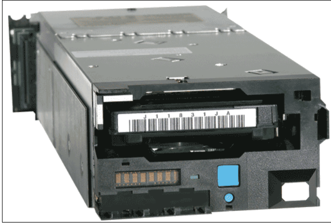
Figure 8-13 IBM TS1120 tape drive
