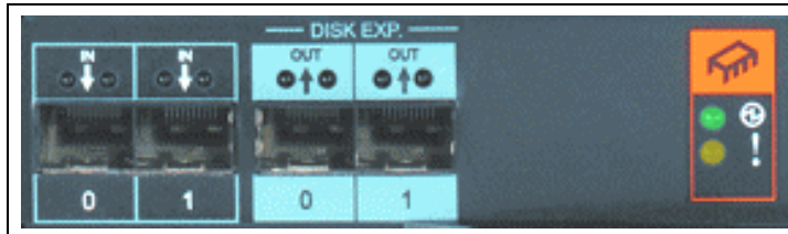
Figure 4-11 SBOD controller card
