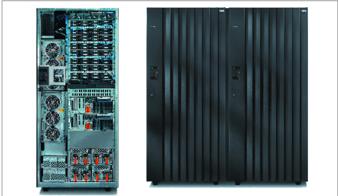
Figure 4-15 DS8000 base frame with covers removed (left) and with Model 94E (right)
