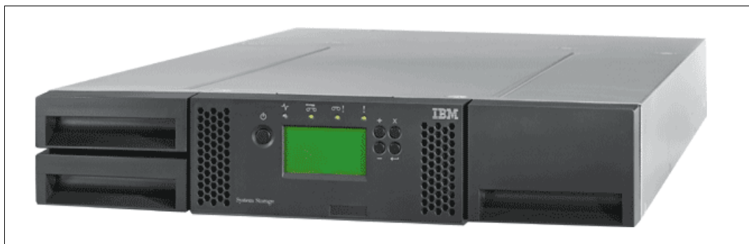
Figure 9-2 IBM System Storage TS3100 Tape Library
