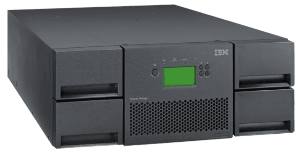
Figure 9-3 IBM System Storage TS3200 Tape Library
