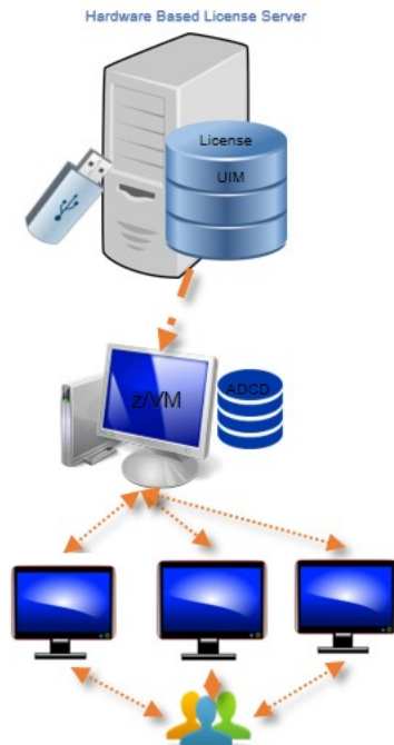
Figure 2. The hardware-based license server and various components of Parallel Sysplex
