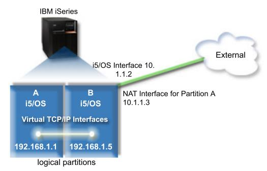
In this example, any existing TCP/IP traffic for the system runs over the 10.1.1.2 interface. A new interface, 10.1.1.3, is created for communicating between the 10.1.1.x network and the 192.168.1.x network. Because this is a static map scenario, the inbound traffic gets translated from the 10.1.1.3 interface to the
