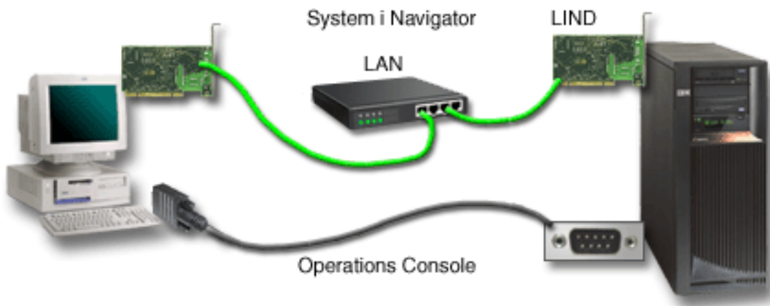
Figure 2. System i Navigator and Operations Console configuration over separate connectivity
