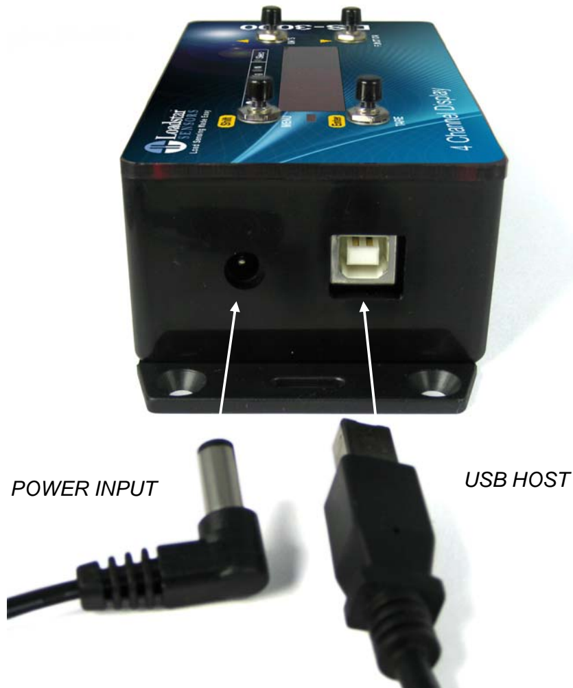
Figure 3: End View: Power and USB Host Connections
