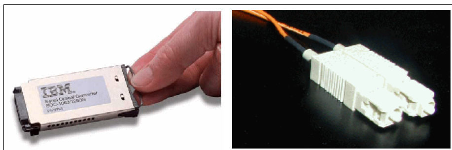
Figure 2-4 GBIC Connector and SC Fibre Connection
