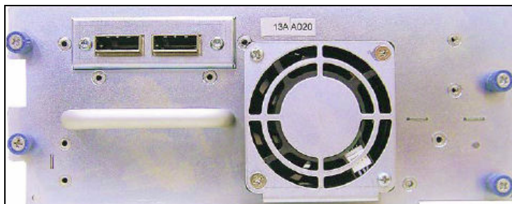
Figure 10-6 The back side of the SAS tape drive
