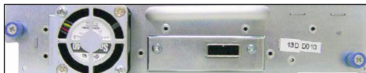
Figure 9-9 Back side of the Half-High SAS Tape Drive
