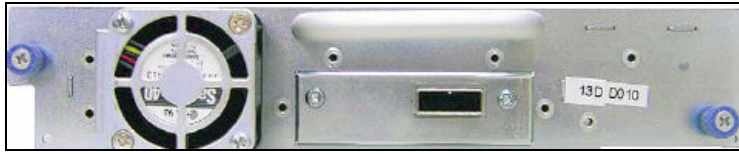
Figure 8-11 The back side of the SAS Half-High Tape Drive
