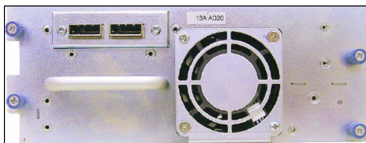
Figure 9-8 Back side of the Full-High SAS Tape Drive
