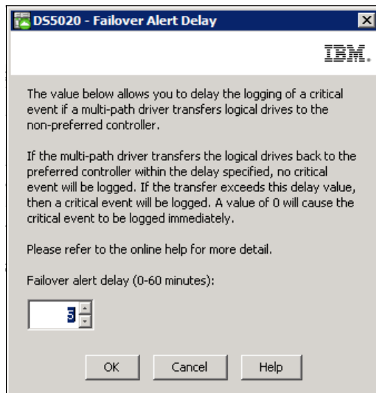
Figure 3-114 Storage subsystem failover alert delay
