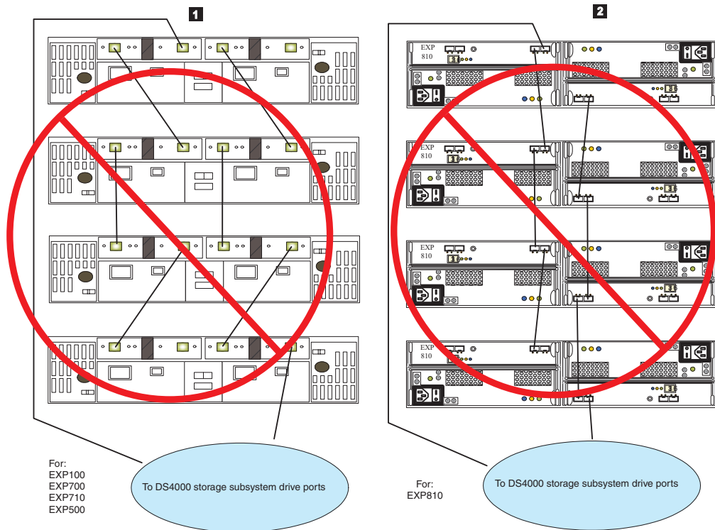
Figure 39. Unsupported cable loop scheme for connecting storage devices (2 of 2)
