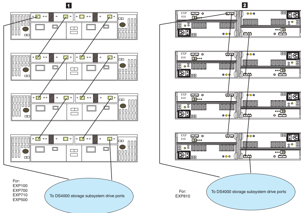
Figure 35. Best practice cable loop scheme for connecting storage devices
