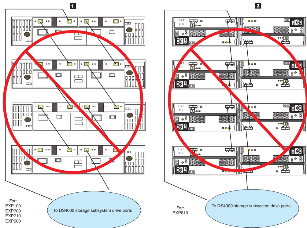
Figure 36. Alternative cable loop scheme for connecting storage devices
