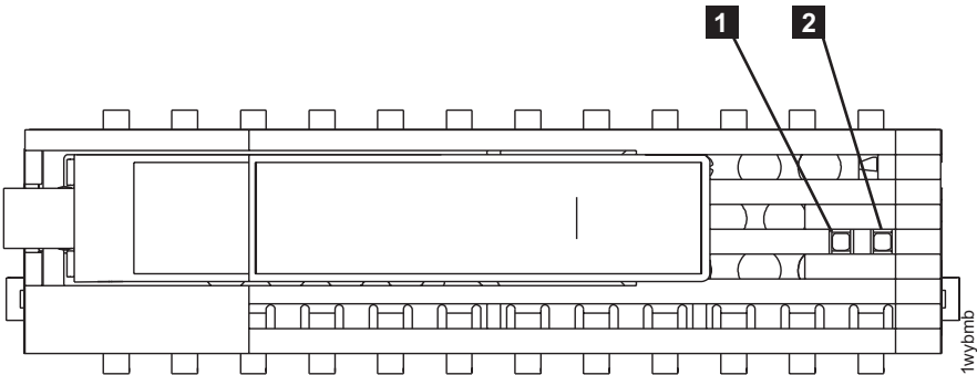
Figure 127. LEDs on a disk drive module (DDM)
