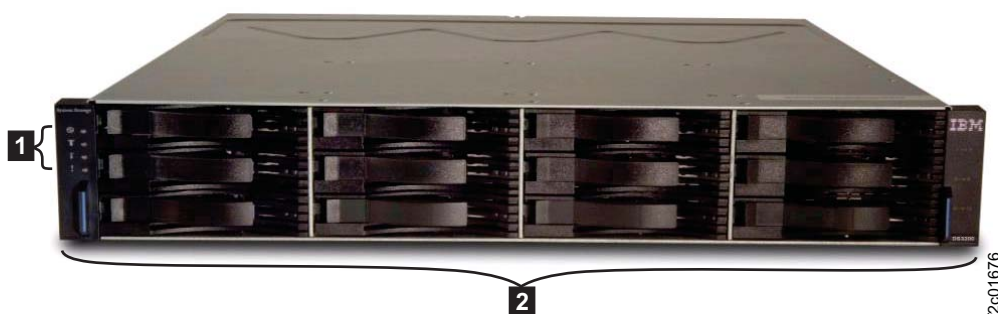
Figure 9. Front view of the LFF storage expansion enclosure
