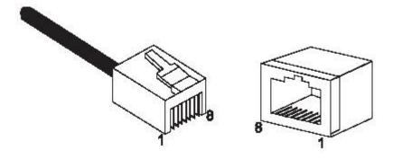
With 10Base-T/100Base-TX cable, pins 1 and 2 are used for transmitting data, and pins 3 and 6 for receiving data. The "+" and "-" signs in the table below are used to represent the polarity of the wires that make up each wire pair.
