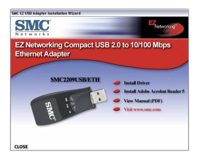
**Step 3:** Please shut down your machine and insert your SMC2209USB/ETH. Once the Windows Operating System is booted up, it will find the new hardware and automatically install it.
