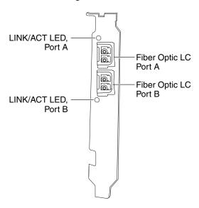
**What the LEDs mean:** The following table explains what the LEDs on this dual-port TOE NIC mean.
