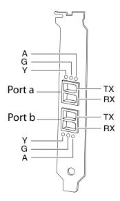
**What the LEDs mean:** The following table explains what the LEDs on the HBA mean.
