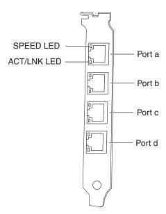
**What the copper GbE NIC LEDs mean:** The following table explains what the LEDs on a multiport GbE NIC mean.
