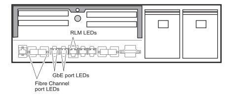
**What the LEDs mean:** The following table explains what the LEDs for your onboard ports mean.
