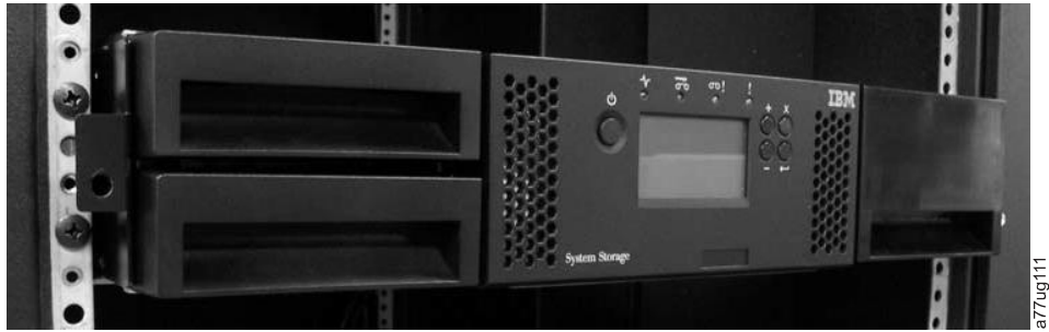
Figure 4-12. Sliding the 2U library into the rack
