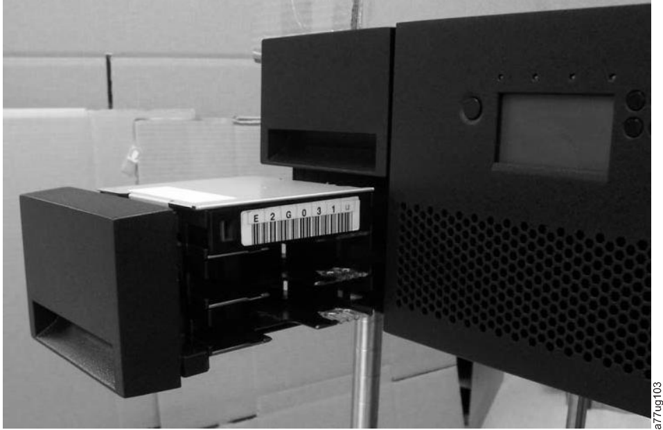
Figure 4-40. 4U library I/O Station in the lower left magazine
