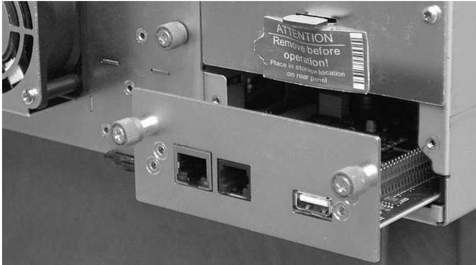
Figure 10-21. Removing a Library Controller Card from the library
