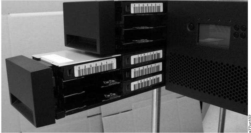
Figure 10-25. Left magazines pulled out of a 4U library (facing front of library)
