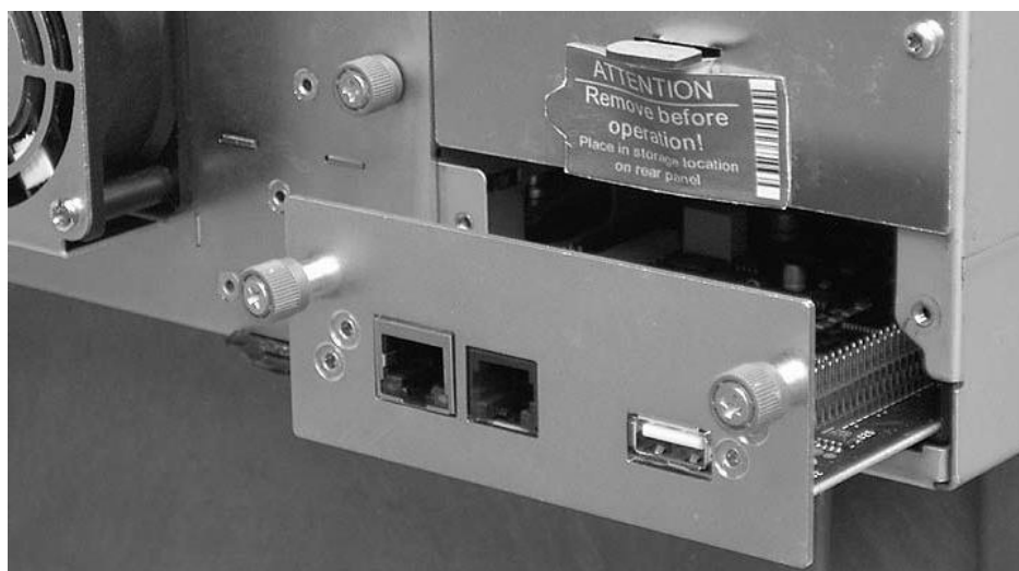
Figure 10-13. A Library Controller Card being removed from the library
