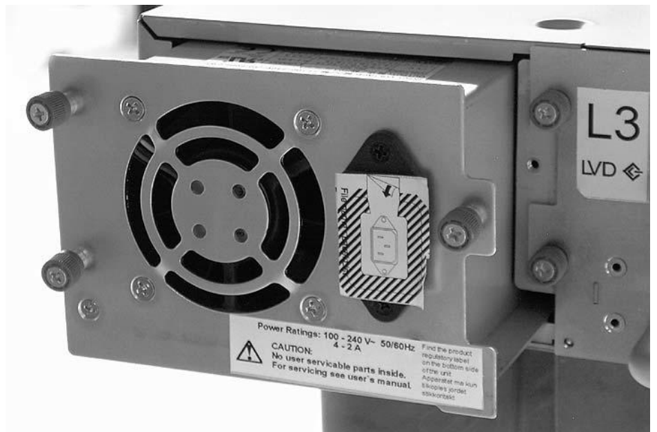
Figure 10-26. A power supply being removed from a library
