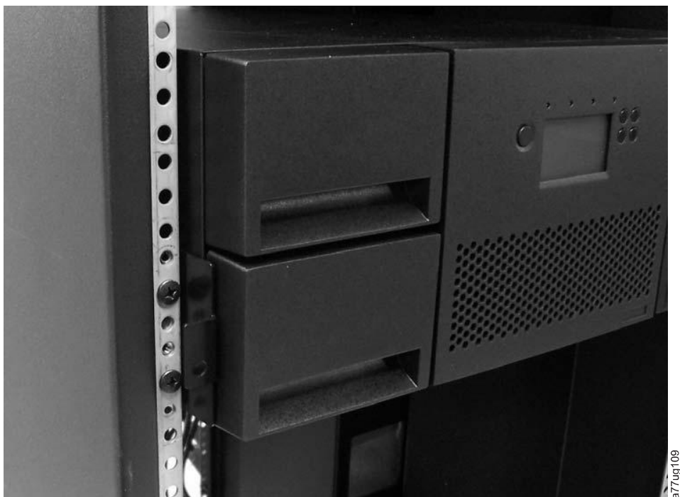
Figure 4-13. Sliding the 4U library into the rack
