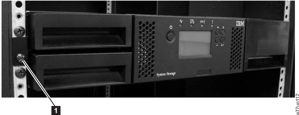
Figure 10-15. Removing the two mounting bracket screws anchoring the library to the rack (one screw on each side of the library)
