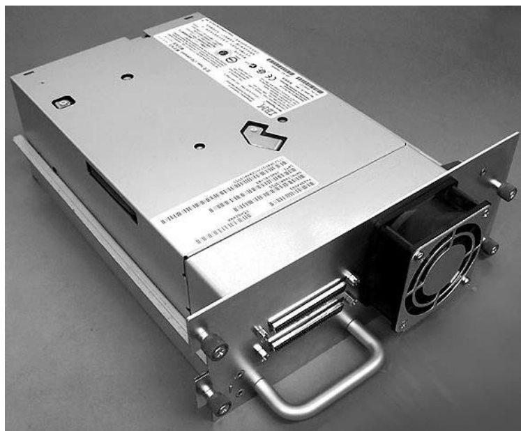
Figure 10-4. Library drive sled without ElectroStatic Discharge (ESD) springs (SCSI sled shown)
