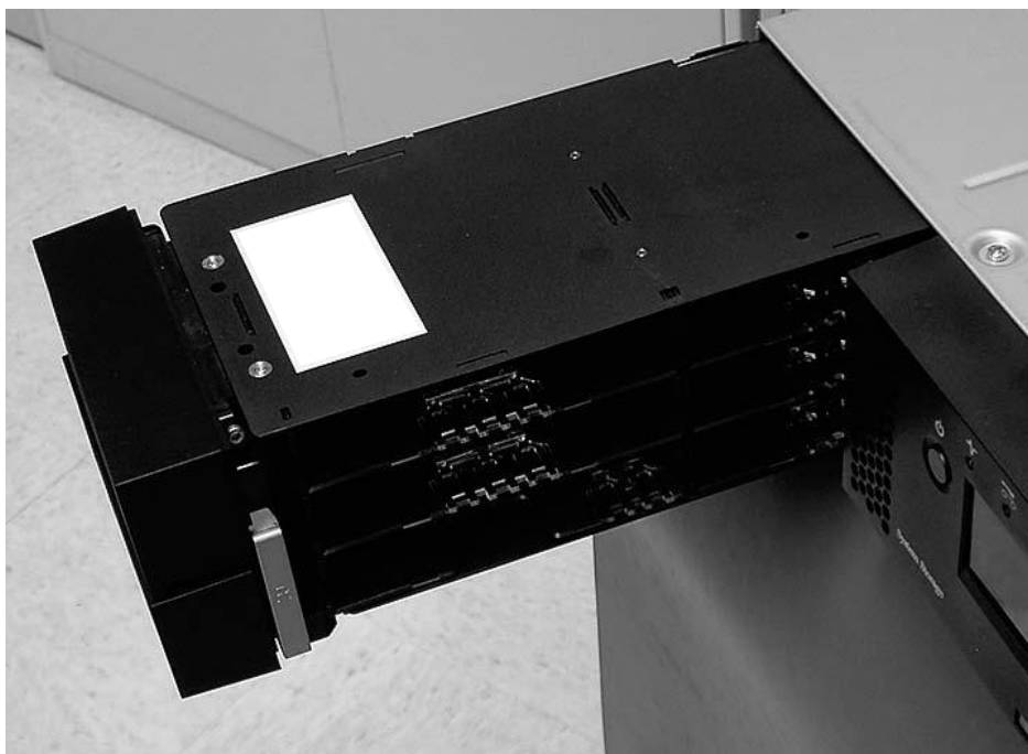
Figure 9-3. Left Magazine pulled out of the 2U Library
