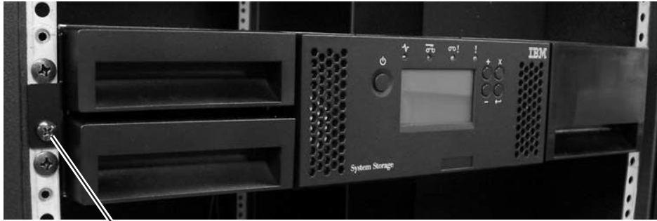
Figure 4-14. Securing the 2U library to the rack
