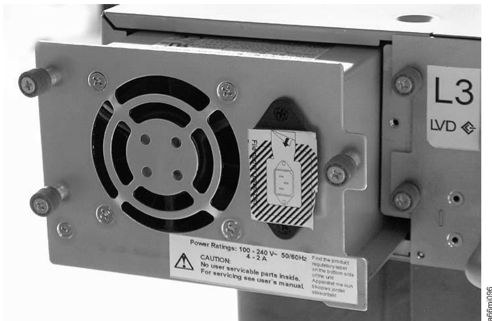
Figure 10-12. A power supply being removed from a 2U library
