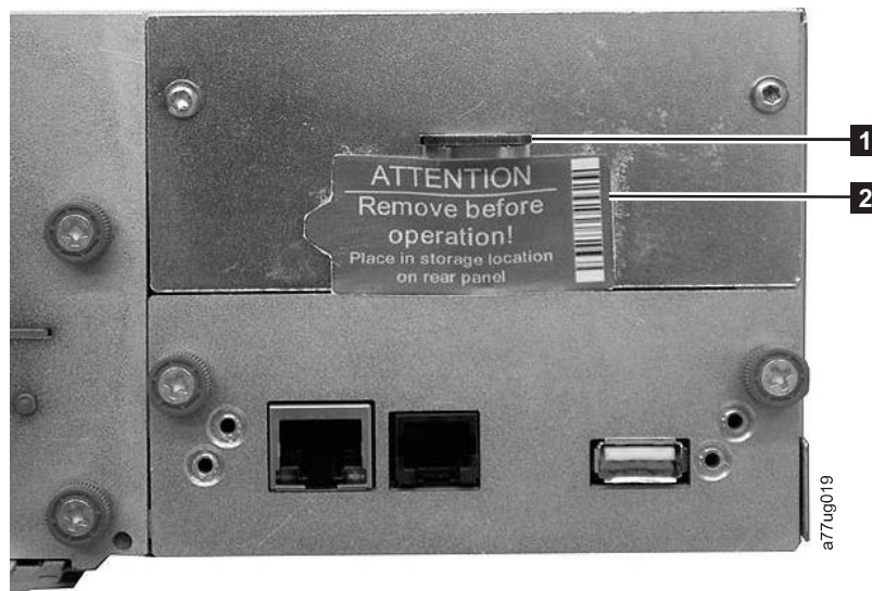
Figure 10-18. Library shipping lock and label storage location on the rear panel of the library
