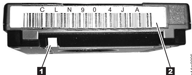
Figure 62. Characteristics that identify the 3592 cleaning cartridge
