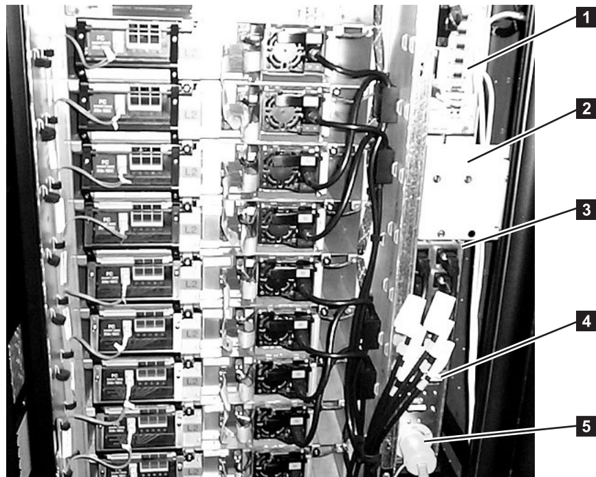
Figure 74. Components of the frame control assembly. Located at the right rear of the TS3500 Tape Library, this power structure comes with models L22, D22, L32, D32, L52, and D52. A model L52 frame is shown.
