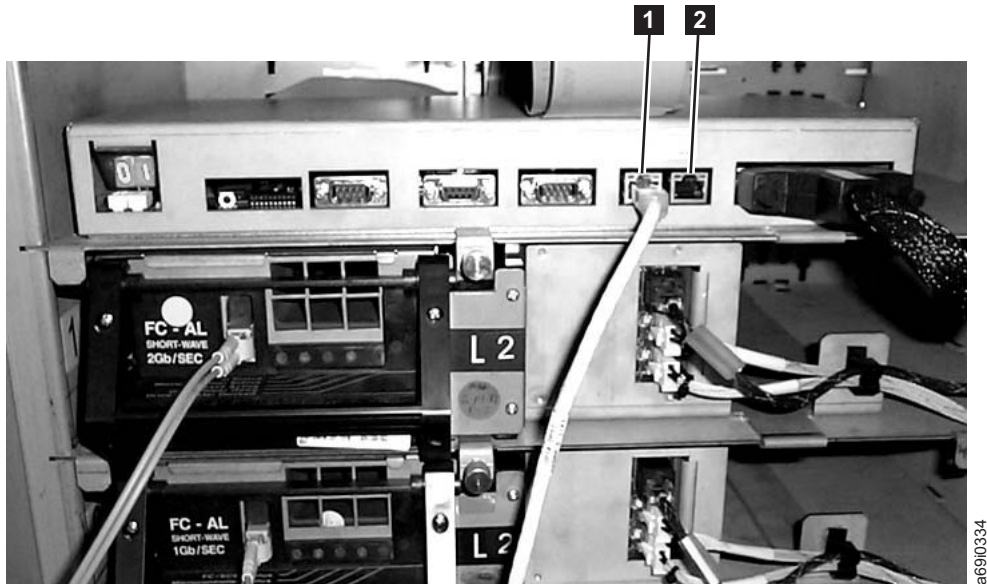
Figure 85. Medium changer assembly. The MCA is located above the drives and the power trays, and is part of the enhanced frame control assembly power structure.
