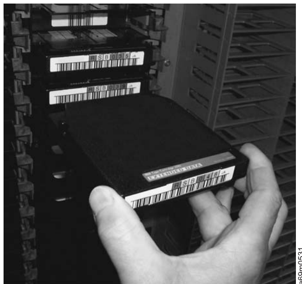
Figure 43. 3592 cartridge removed from an HD slot
