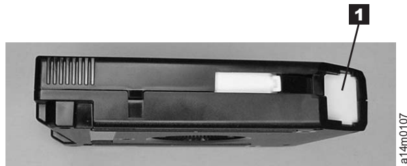
Figure 63. Door of the 3592 cleaning cartridge
