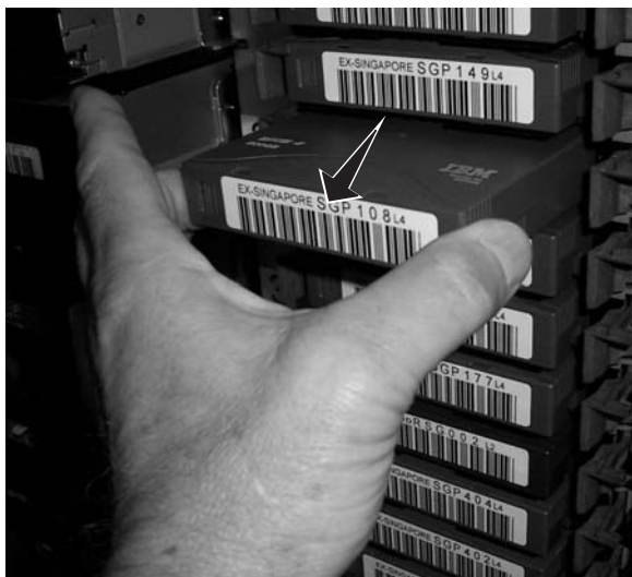
Figure 39. LTO cartridge removal from an HD slot
