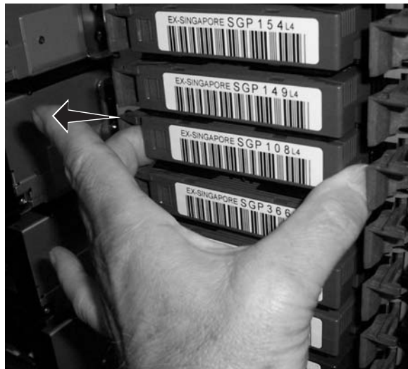
Figure 38. LTO HD slot gate release
