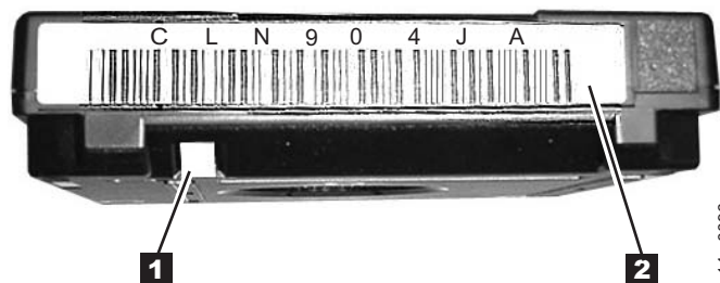
Figure 62. Characteristics that identify the 3592 cleaning cartridge
