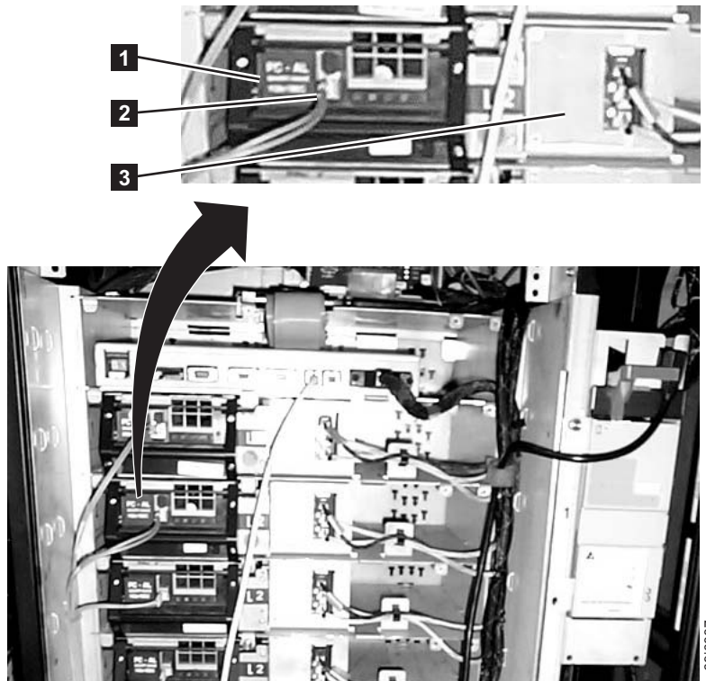
Figure 88. Compartment that houses the tape drives and the fixed tray assemblies in Model L53 or D53 frames. The view is from the rear of the TS3500 Tape Library. Only the items designated in the preceding list are customer accessible. All other items are for service personnel.
