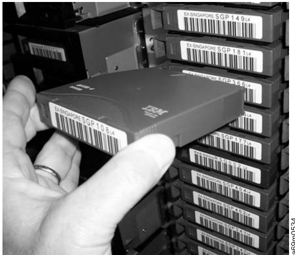
Figure 40. LTO cartridge removed from an HD slot
