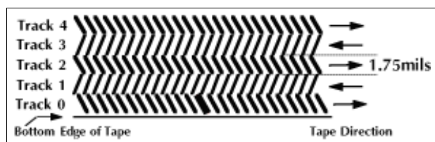
Figure 1-12 Symmetric Phase Recording technology
