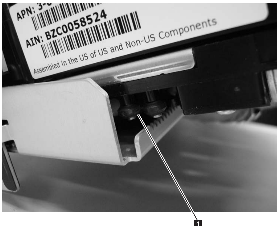
Figure 8-96. Align rollers on the Picker Assembly with slots on the M2 Robot Assembly
