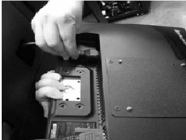
Figure 18. Connect the power cord to the monitor
