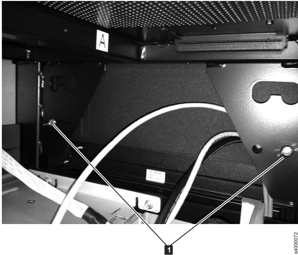
Figure 5. Wing screws securing the side panel
