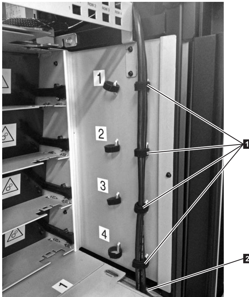
Figure 26. Power cords secured with hook and loop fasteners
