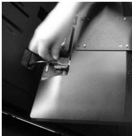
Figure 17. Connect the VGA cable to the monitor
