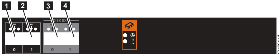
Figure 23. Expansion enclosure processor card port location codes
