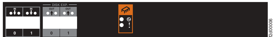
Figure 10. Expansion enclosure processor card indicators
