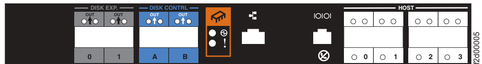
Figure 9. Server enclosure processor card indicators
