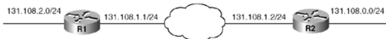
Figure 9-32. Network Setup to Produce Stuck in EXSTART/EXCHANGE Problem
