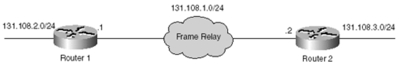
Figure 3-27. NBMA Frame Relay Network Vulnerable to Broken Multicast Capability Problems
