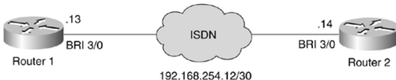
Figure 3-44. Network Setup Vulnerable to DDR Problems
