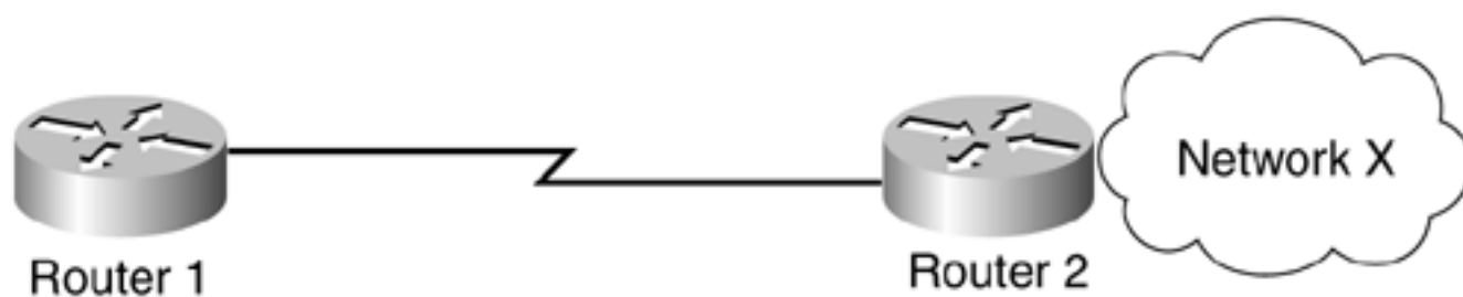
Figure 4-2. An Example of the Split Horizon Technique
