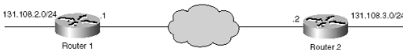
Figure 3-13. Two Routers Running RIP in a Frame Relay Environment
