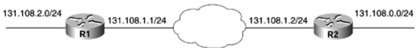
Figure 9-66. OSPF Network Setup Used to Produce Route Installation Problems
