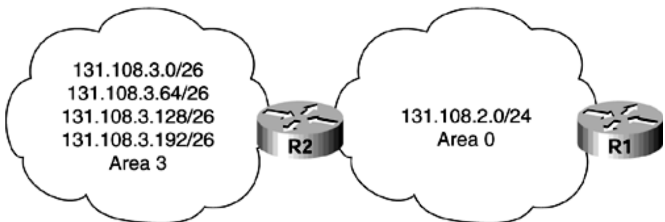
Figure 9-83. OSPF Network in Which a Router Is Not Summarizing Interarea Routes
