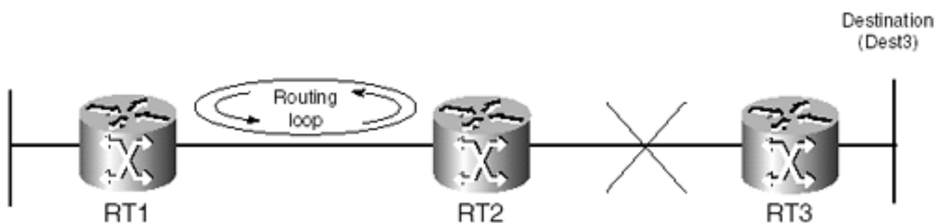
Figure 1-10. Routing Loops in Distance Vector Environments
