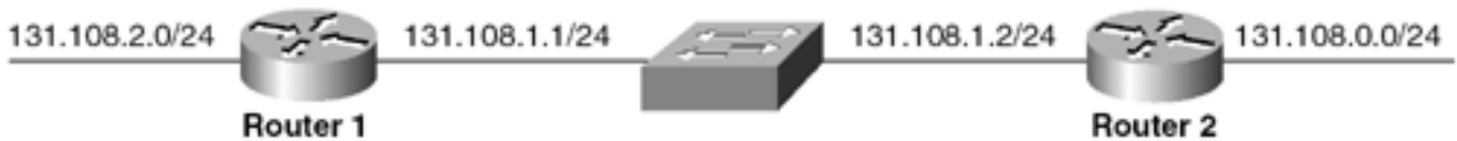
Figure 9-24. Network Setup Vulnerable to OSPF Neighbor Stuck in INIT Problem Because of Broken Multicast Capabilities
