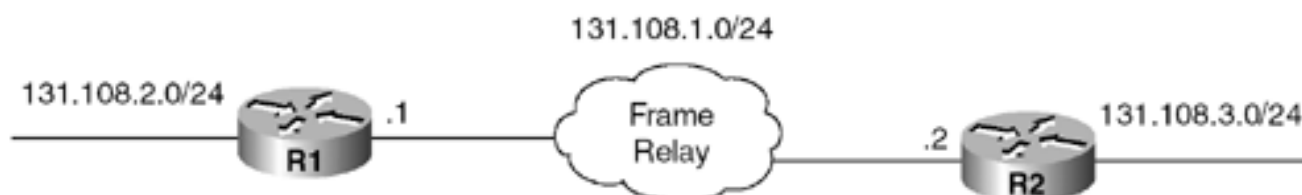
Figure 9-27. Network Topology Used to Produce OSPF Neighbor Stuck in INIT Problem
