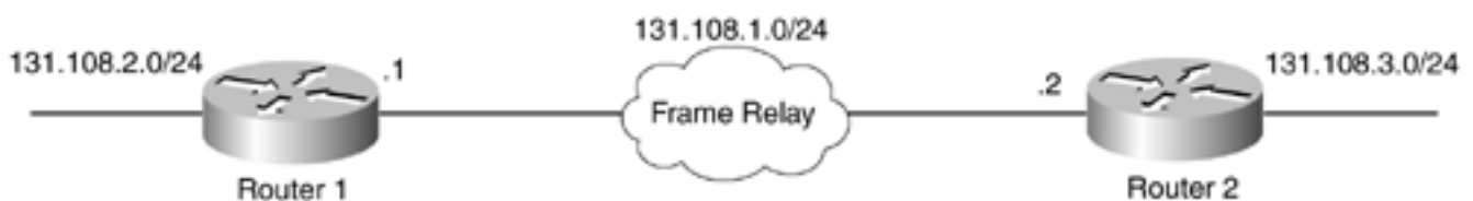
Figure 5-22. Network Setup Incompatible with Frame Relay Broadcasting Without broadcast Keyword in map Statement
