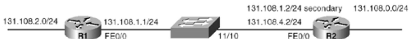
Figure 9-12. Two Routers Connected Through a Switch, with One Side's Primary Interface IP Address Identical to the Other Side's Secondary
