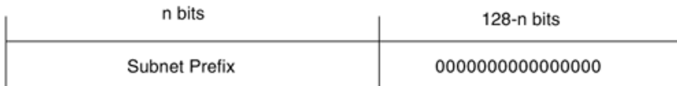
Figure 8-7. Subnet-Router Anycast Address
