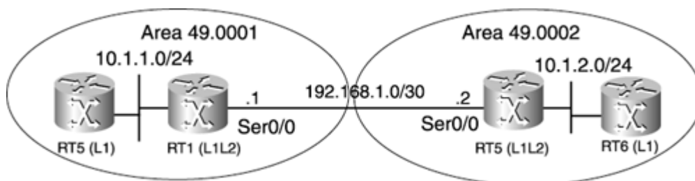
Figure 11-11. Basic Network for Testing Operation of the ping clns and traceroute clns Commands
