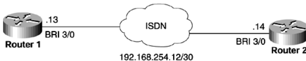
Figure 9-89. OSPF Network Experiencing a Perpetual DDR Link Problem
