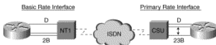
Figure 11-5: Connectivity to ISDN using BRI and PRI.
