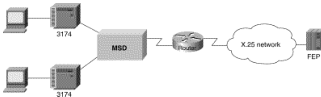
Figure 5-20: QLLC conversion supports multidrop SDLC topology.
