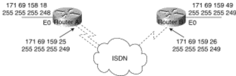
Figure 10-7: Example of dial backup over ISDN.
