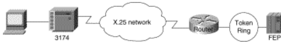
Figure 5-18: Simple topology for QLLC conversion.
