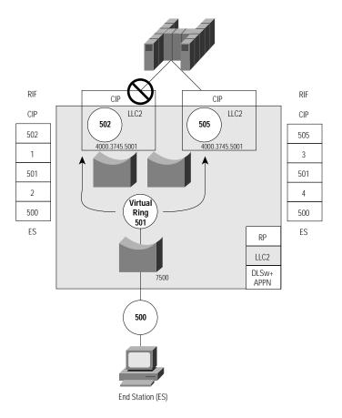
Figure 2-10 **Using Duplicate MAC Addresses with CIPs**
