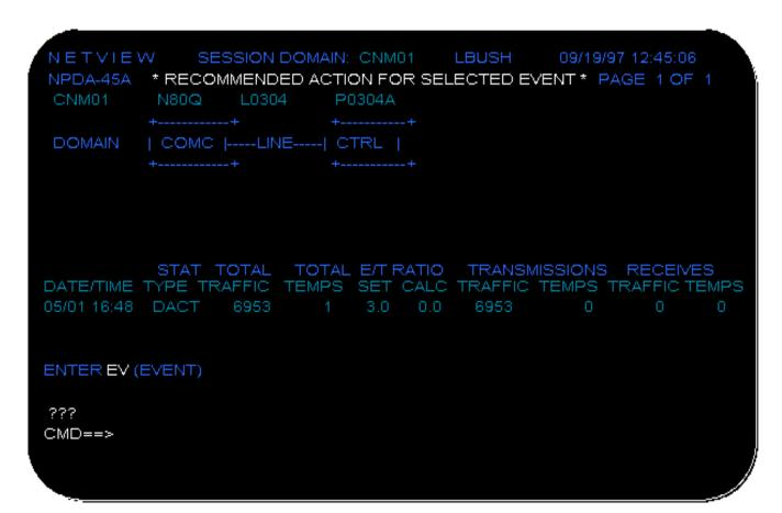
Native Service Point provides the ability to collect statistics based on user-defined intervals. Router CPU and memory utilization data is collected and archived. Interface statistics also can be collected and archived. Figure 4-5 shows an example of records collected for an Native Service Point-managed interface.
