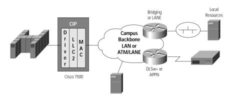
Figure 1-5 **Connecting Local Resources to the CIP**
