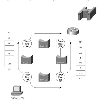
Figure 2-9 **Explorer Processing on a Source-Route Bridged LAN**
