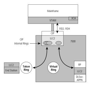
The CIP running CSNA will support multiple internal LAN interfaces, each of which looks like a LAN port to VTAM. (VTAM supports a maximum of 18 LAN ports.) However, only a single LAN port is required. CSNA also supports up to 256 open LLC2 SAPs per LAN port.
