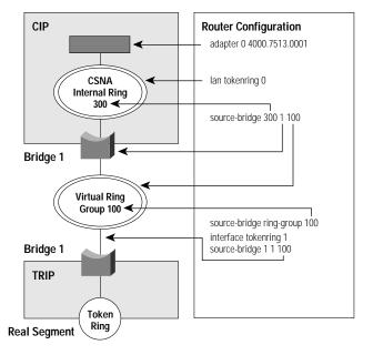
Figure 3-2 **Using Virtual Rings to Provide Connectivity**
