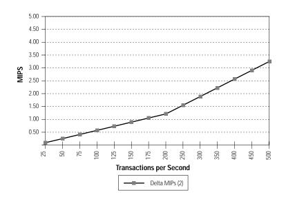
Figure 2-3 Impact on a 9121-982 Mainframe of Migrating from a FEP to a CIP
