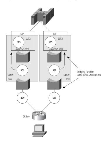
Figure 2-12 Load Balancing Using Duplicate MAC Addresses and DLSw+
