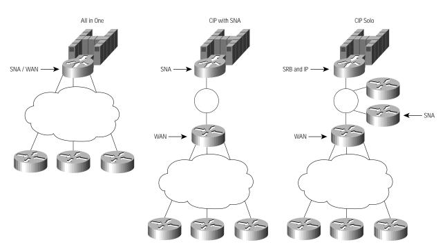
Figure 2-2 **Alternatives for Functionality Placement**
