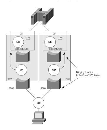
Figure 2-11 Load Balancing Using Duplicate MAC Addresses and SRB
