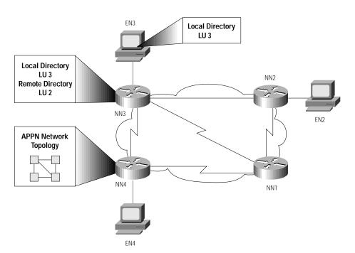
Figure 1-2 Sample APPN Network and Associated Directory and Topology Databases
