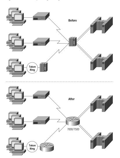
Figure 3-8 Replacing a Single FEP with a Channel-Attached Router
