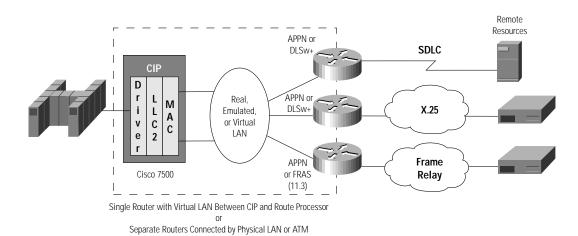
Figure 1-7 Connecting Remote SNA Devices over SDLC, X.25, or Frame Relay
