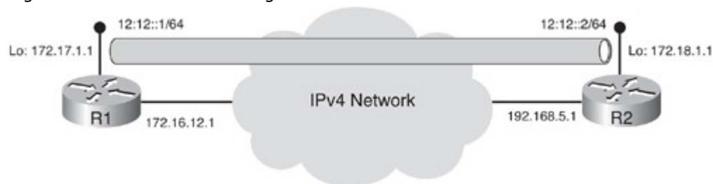
Figure 8-41. Tunnel Connecting IPv6 Networks over an IPv4 Network.
