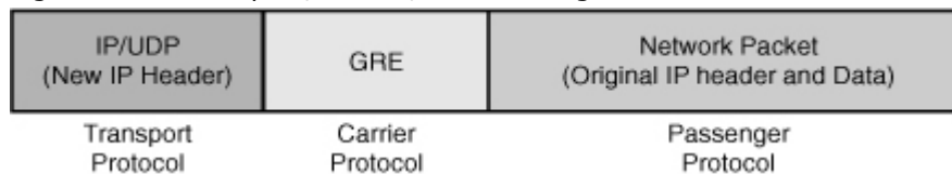
Figure 7-22. Transport, Carrier, and Passenger Protocols.
