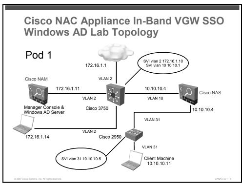
The figure shows the topology of the in-band VGW SSO Windows Active Directory Cisco NAC Appliance lab.
