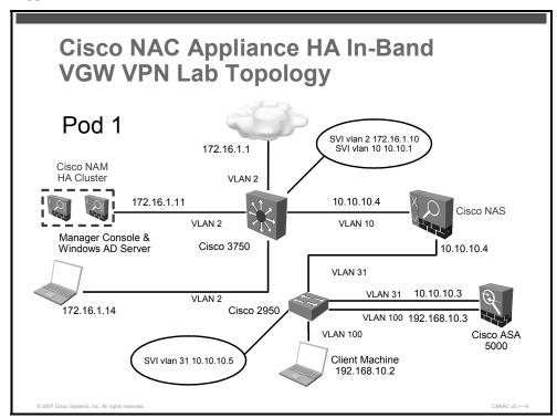
The figure shows the topology for the Cisco NAM HA cluster, a part of the highly available inband VGW VPN Cisco NAC Appliance lab.
