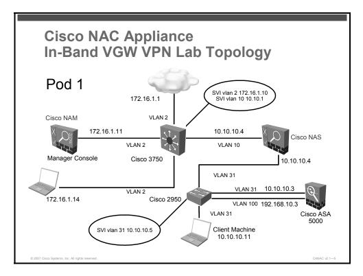
The figure shows the topology of the in-band VGW VPN Cisco NAC Appliance lab.
