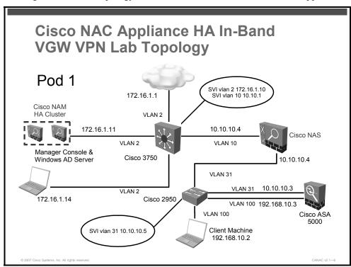
The figure shows the topology for the HA in-band VGW VPN Cisco NAC Appliance lab.
