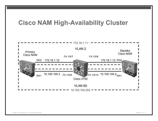
The figure shows the topology for the Cisco NAM HA cluster, a part of the HA out-of-band VGW Cisco NAC Appliance lab.
