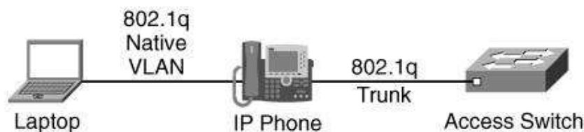
Figure 12-6. IP Phone with a Built-In Switch Connects to the Access Switch and User's Laptop
