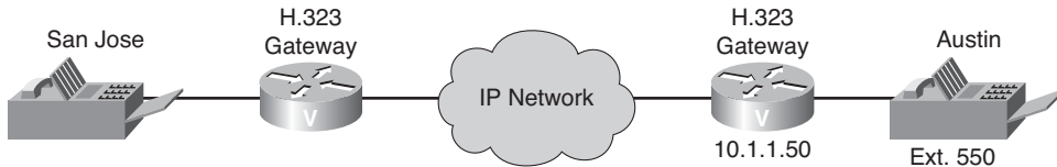
Figure 5-13 H.323 Fax Pass-Through Configuration Example Topology
