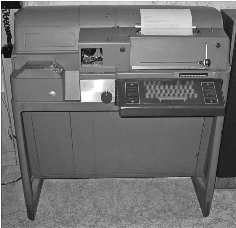
Figure 3-1 1950 Era Model 28 TTY by Teletype Corporation
