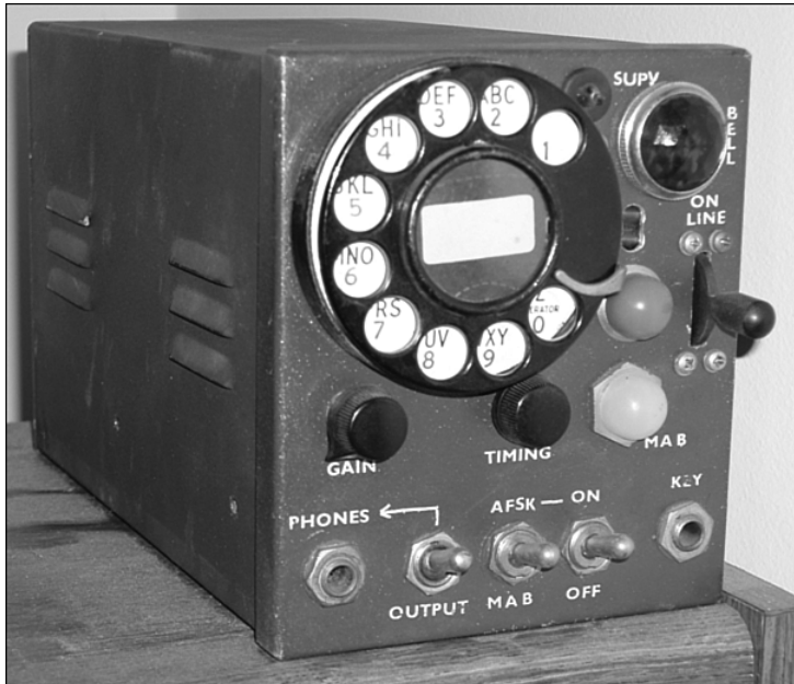
Figure 3-2 Robert Weitbrecht's First Modem, Courtesy of Jim Haynes
