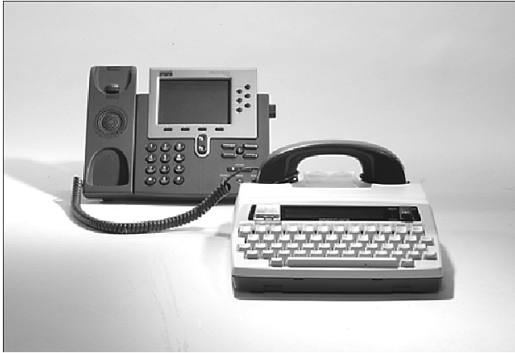
Figure 3-5 Text Telephone with an Acoustic Coupler Connected to a Cisco IP Phone
