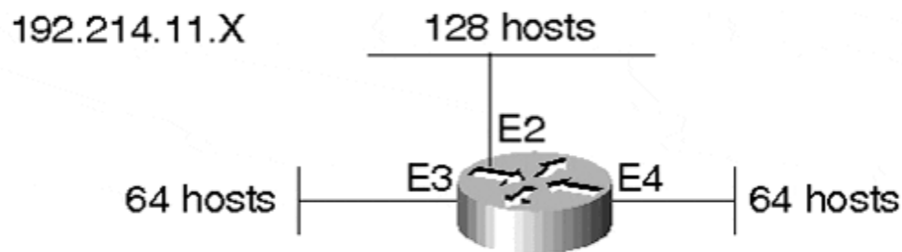
Figure 3-7. Example of a Class C Network Divided into Three Subnets
