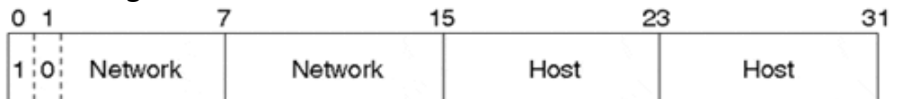
Figure 3-2. General Class B Address Format
