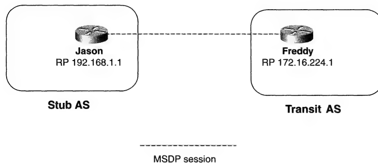
Figure 7-18 BGP Is Typically Not Run Between a Stub AS and Its Transit AS, but This Can Cause a Problem for MSDP
