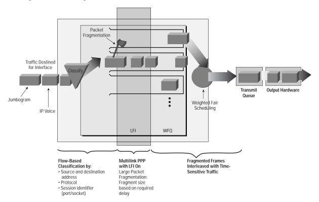
LFI was designed especially for lower-speed links where serialization delay is significant. LFI requires that multilink PPP be configured on the interface with interleaving turned on. A related IETF Draft, called Multiclass Extensions to Multilink PPP (MCML) implements almost the same function as LFI.
