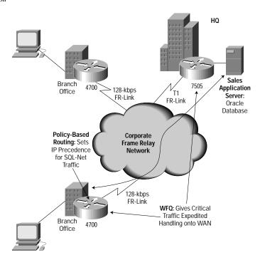
To implement this policy, the company uses WFQ with IP Precedence signaling to ensure that data to the sales application receives the network resource it needs, while ensuring that other WAN users also receive service, albeit slightly less timely if the sales application is being used heavily.
