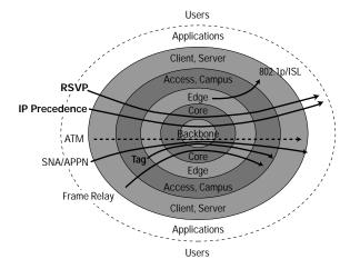
Cisco IOS software takes advantage of the end-to-end nature of IP to meet this challenge by overlaying Layer 2 technology-specific QoS signaling solutions with the Layer 3 IP QoS signaling methods of RSVP and IP Precedence.
