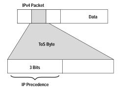
Features such as policy-based routing and CAR can be used to set precedence based on extended access-list classification. This allows considerable flexibility for precedence assignment, including assignment by application or user, or by destination and source subnet, and so on. Typically this functionality is deployed as close to the edge of the network (or administrative domain) as possible, so that each subsequent network element can provide service based on the determined policy.
