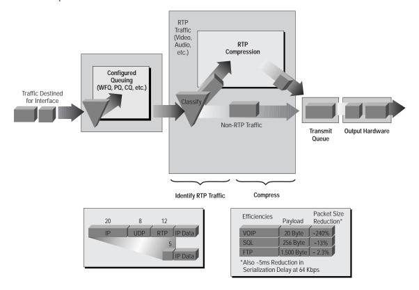
RTP header compression is supported on serial lines using Frame Relay, HDLC, or PPP encapsulation. It is also supported over ISDN interfaces. A related IETF Draft, called Compressed RTP (CRTP), defines essentially the same functionality.
