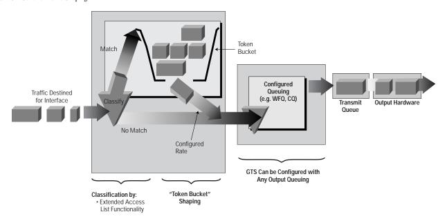
GTS applies on a per-interface basis, can use access lists to select the traffic to shape, and works with a variety of Layer 2 technologies, including Frame Relay, ATM, Switched Multimegabit Data Service (SMDS), and Ethernet.
