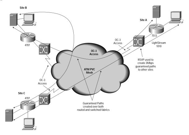
In this instance, OC-3 ATM links are configured with multiple 3 Mbps PVCs connecting to various remote sites. RSVP ensures that QoS from this PVC is extended to the appropriate application across the local routed network. In the future, Cisco IOS will extend this RSVP capability to dynamically set up ATM SVCs. This will reduce configuration complexity and add a great degree of automatic configuration.
