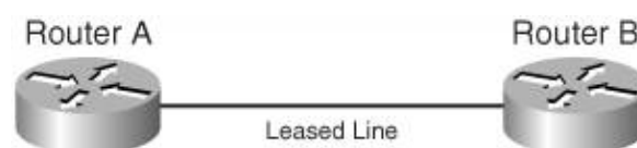
Figure 8-5. One Leased Line Connecting Two Routers
