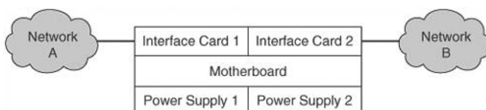
Figure A-1. Calculating Availability for a Simple System
