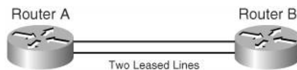
Figure 8-6. Two Leased Lines Connecting Two Routers
