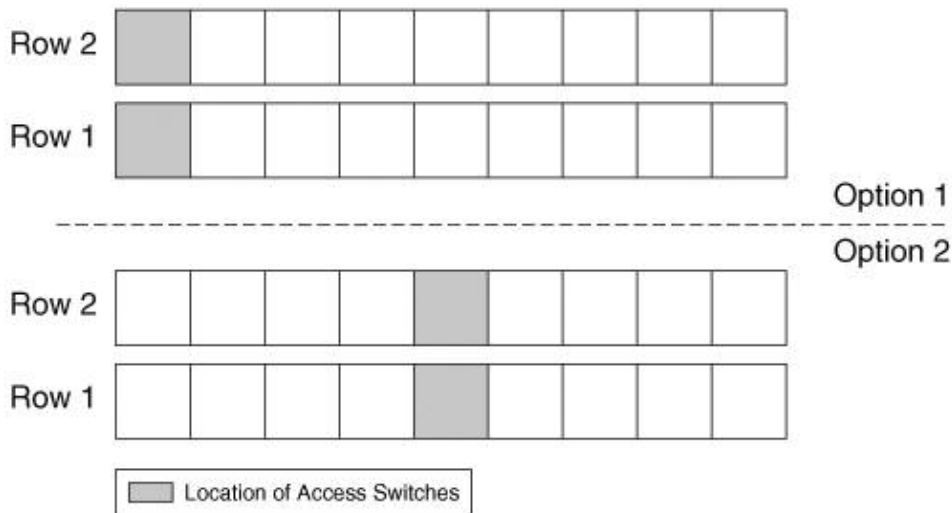
Figure 9-8. Possible Locations of Access Switches
