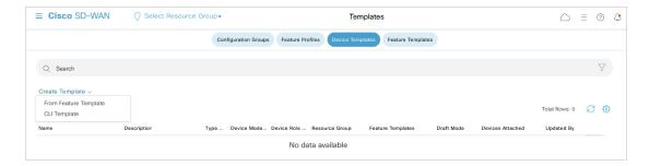
A device template consists of several feature templates. Each feature template defines the configuration for a particular Cisco SD-
