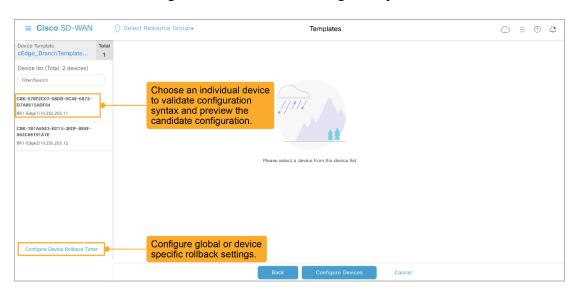
In the case of a serious misconfiguration, such as a wrong interface address or a missing defa ult route, you may lose the control connection to the WAN Edge router. All Cisco WAN Edge devices are configured with a rollback function. If a device loses control connections after a configuration, it can automatically roll back to the previous configuration. The rollback timer can be configured at the bottom left of the screen.
