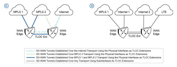
Figure C shows TLOC Extensions on separate physical interfaces while Figure D shows multiple TLOC extensions using subinterfaces across two physical interfaces.
