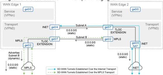
Some routing considerations need to take place for controller reachability to occur and for IPsec tunnels and BFD sessions to come up with other sites over the TLOC extension interfaces. Static default routes should be configured in the underlay (transport VPN 0) on each WAN Edge router, pointing to the service provider router as the next hop.
