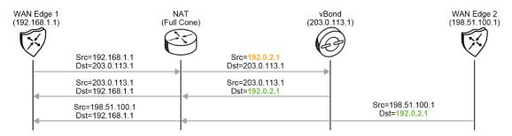
Full-cone NAT is also known as one-to-one NAT. You can use full-cone NAT to map an internal address and port pair with an external address and port.
