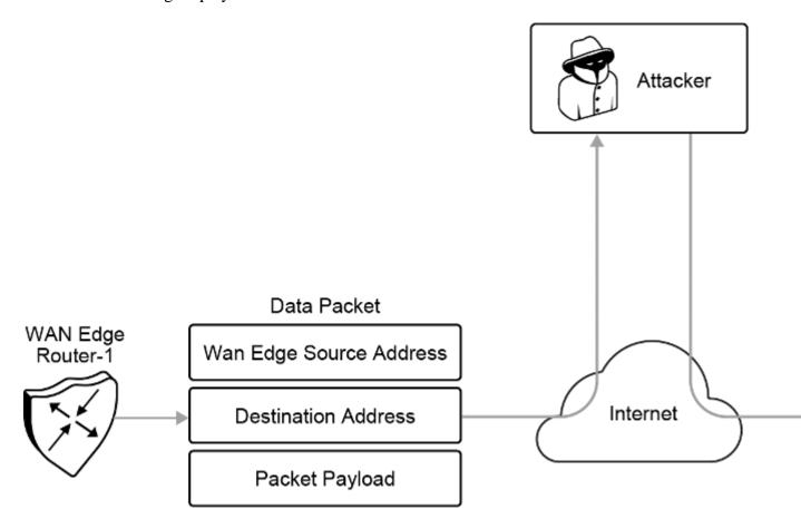
• **Sliding Window Mechanism**: Cisco SD-WAN uses a **sliding window** to define the range of acceptable sequence numbers. If a packet's sequence number is outside this range or a
