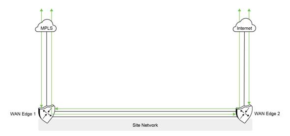
In the figure, WAN Edge 1 connects directly to the MPLS transport and uses the TLOC extension interface on WAN Edge 2 to connect to the internet transport. In turn, WAN
