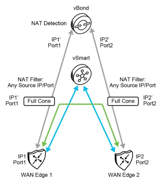
WAN Edge router establishes initial connection with the vBond orchestrator at bootup.
