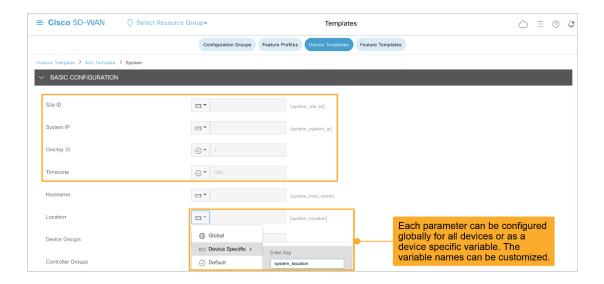
If you select the device-specific option, you can adapt the variable names to potentially already existing variables in other components in a software-defined environment. Unless there is a good reason, the recommendation is to not change those variable names.
