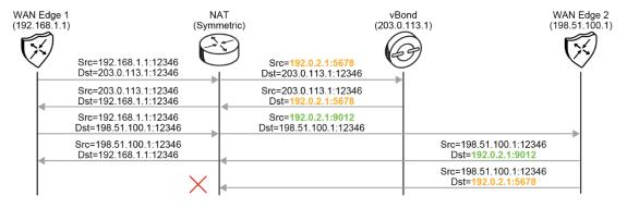
With the symmetric NAT method, each request from the same internal socket to a specific destination socket is
