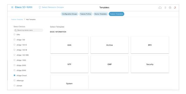
A feature template is used for each feature of a device configuration, which explains the high number of templates that are displayed in
