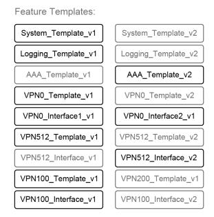
When working with templates, it is important to remember whether you are looking at a device or a feature template and how they fit together. A simple analogy would be that of a puzzle. The feature templates are the individual puzzle pieces that come together to form the complete puzzle (that is, the device template).
