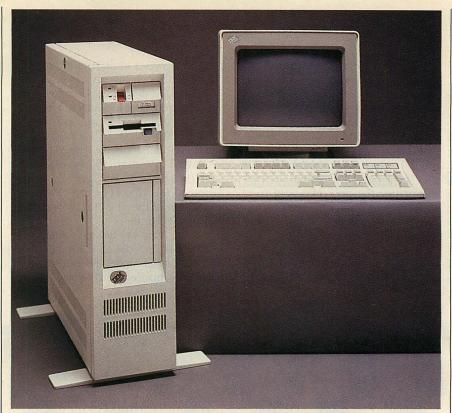
The IBM PS/2 Model 80, Type 8580-111, is a floor-standing unit with a separate display and keyboard. It comes standard with a 20-MHz 80386, 2MB of RAM, and a 115MB hard disk. An optional 70MB, 115MB, or 314MB hard disk can be added.
