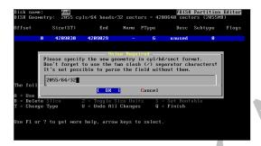
3 To calculate the correct geometry, find the total number of sectors by multiplying the number of cylinders, heads and sectors per head together, and then dividing the number of sectors by the correct number of heads and sectors per head.
