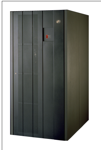
Figure A-5 9672 Parallel Enterprise Server
