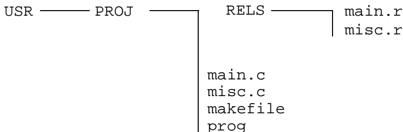
Figure 4-2 I-Code Linking Makefile Example Directory Structure
