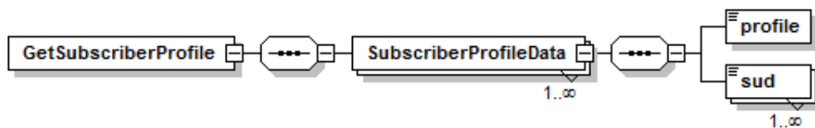
Figure 1 Parameters in Get Response Subscriber Profile
