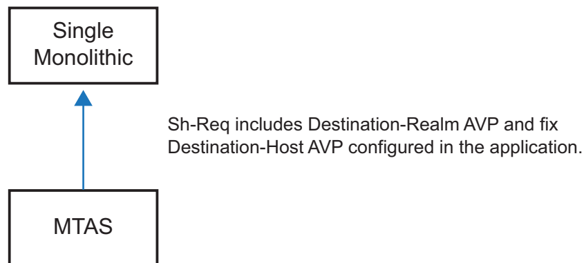
Figure 1 Layout of Classic Single Network Architecture
