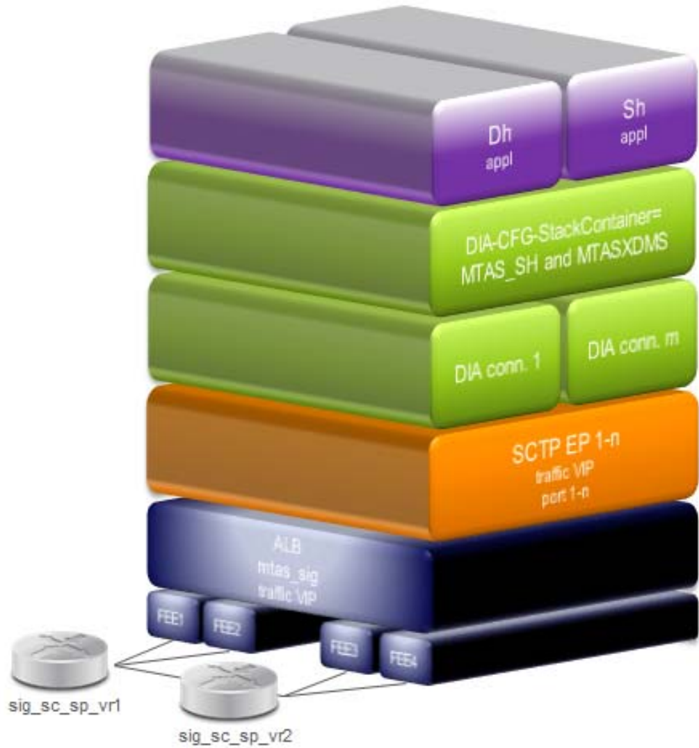
Figure 2 Dh/Sh in MTAS, The Interface Is Bound to a Single-Homed Local SCTP EndPoint
