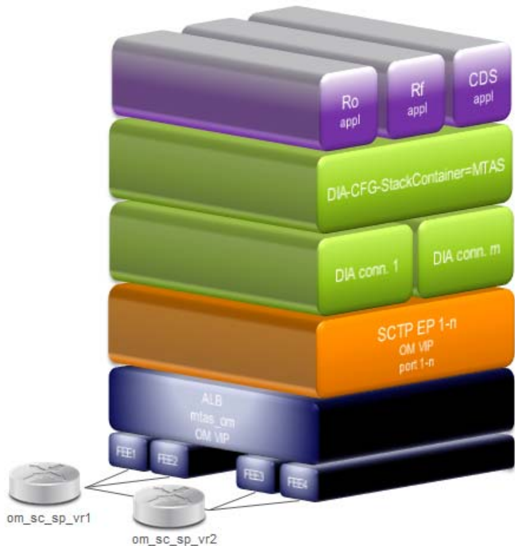
Figure 3 Rf/Ro/CDS in MTAS, The Interface Is Bound to a Single-Homed Local SCTP EndPoint
